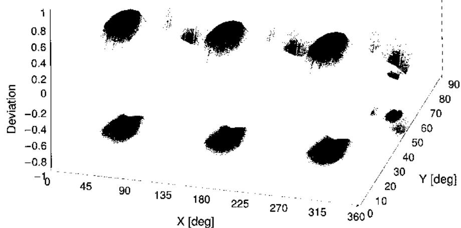
60GHz: 3D isotropy, E-field parallel to probe axis
