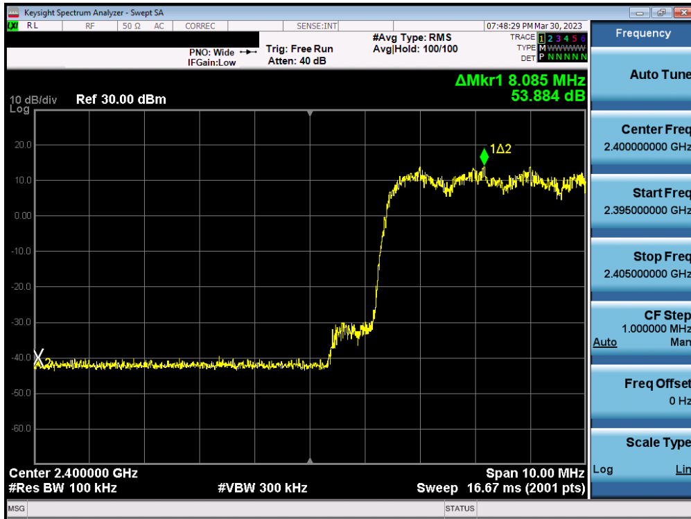
Plot 7-33. Band Edge Plot Ant2 (Bluetooth with Hopping Enabled, 8DPSK, ePA, 2.4GHz)
