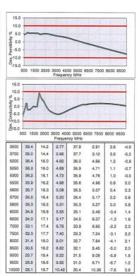
Figure D-2 600 - 10000 MHz Head Tissue Equivalent Matter
