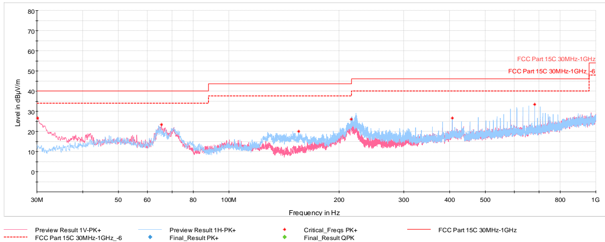
Plot 7-627. Radiated Spurious Emissions below 1GHz CDD 11ax - SU Ch.6, with AC/DC Adapter
