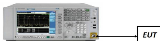
Figure 7-5. Test Instrument & Measurement Setup
