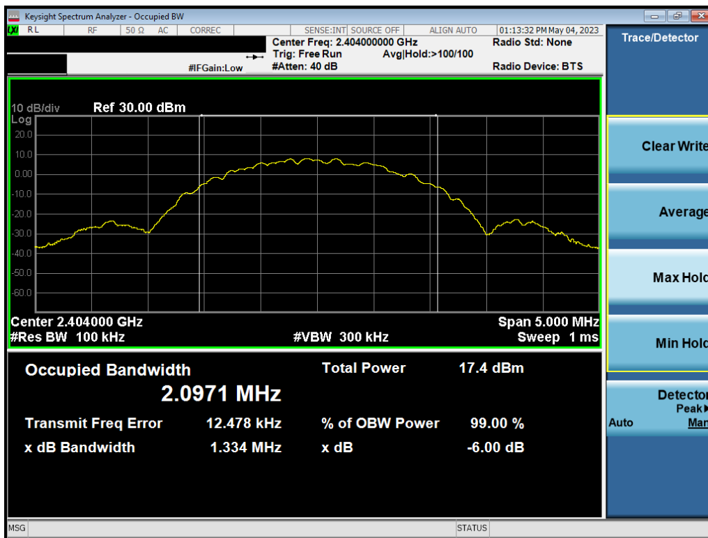
Plot 7-10. 6dB BW & 99% OBW Plot Ant2 (Bluetooth (LE), 2Mbps, ePA – Ch. 1)
