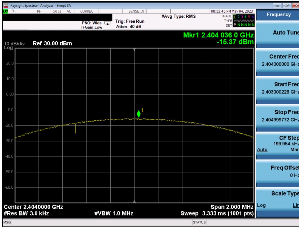
Plot 7-67. Power Spectral Density Plot Ant1 (Bluetooth (LE), 2Mbps, iPA – Ch. 1)
