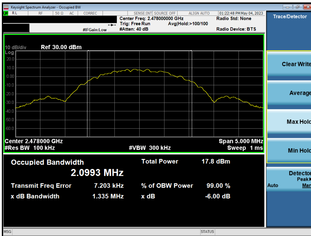
Plot 7-12. 6dB BW & 99% OBW Ant2 (Bluetooth (LE), 2Mbps, ePA – Ch. 38)
