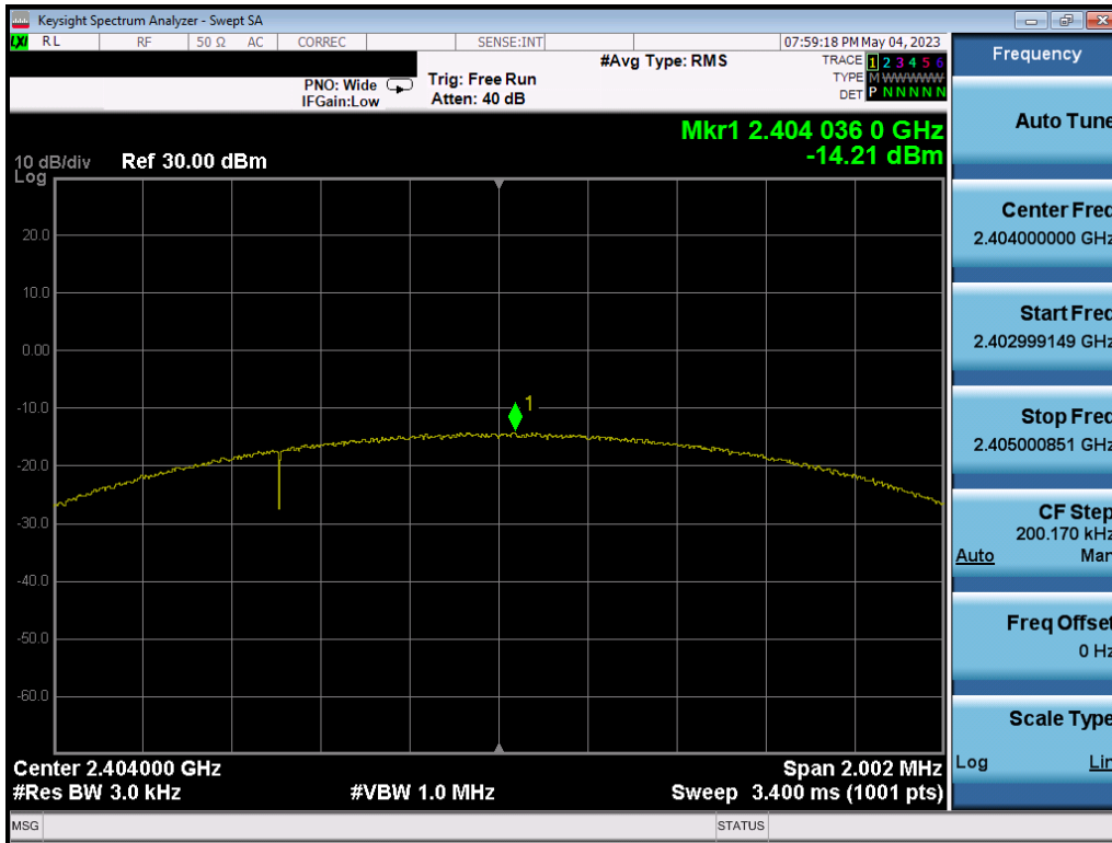
Plot 7-61. Power Spectral Density Plot Ant1 (Bluetooth (LE), 2Mbps, ePA – Ch. 1)
