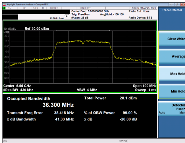
Plot 7-15. 26dB BW & 99% OBW Ant1 (40MHz BW 802.11n – Ch. 110, MCS2)
