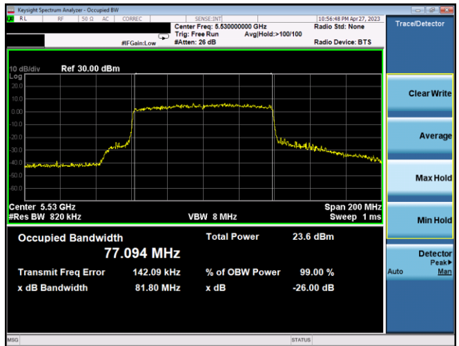
Plot 7-36. 26dB BW & 99% OBW Ant1 (80MHz BW 802.11ax(SU) – Ch. 106, MCS4)
