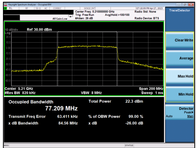
Plot 7-6. 26dB BW & 99% OBW Ant1 (80MHz BW 802.11ax(SU) – Ch. 42, MCS2)
