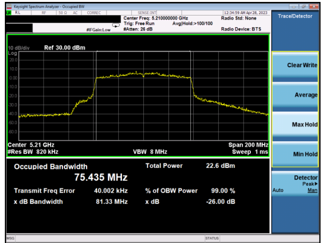
Plot 7-5. 26dB BW & 99% OBW Ant1 (80MHz BW 802.11ac – Ch. 42, MCS2)
