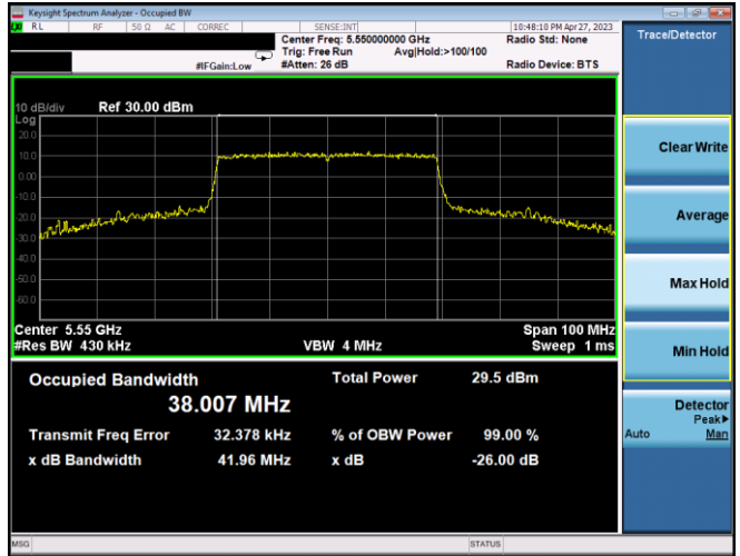
Plot 7-34. 26dB BW & 99% OBW Ant1 (40MHz BW 802.11ax(SU) – Ch. 110, MCS4)
