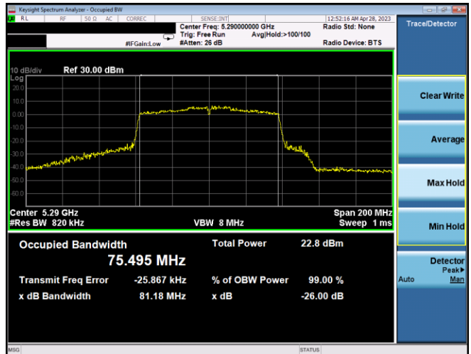
Plot 7-29. 26dB BW & 99% OBW Ant1 (80MHz BW 802.11ac – Ch. 58, MCS4)
