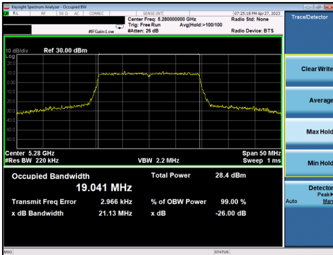
Plot 7-8. 26dB BW & 99% OBW Ant1 (20MHz BW 802.11ax(SU) – Ch. 56, MCS2)
