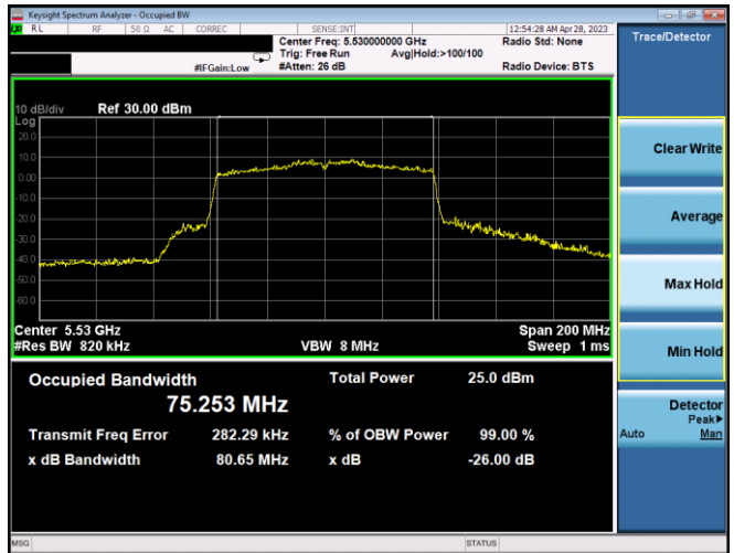
Plot 7-35. 26dB BW & 99% OBW Ant1 (80MHz BW 802.11ac – Ch. 106, MCS4)
