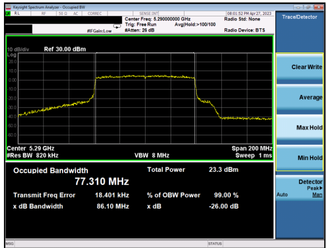
Plot 7-12. 26dB BW & 99% OBW Ant1 (80MHz BW 802.11ax(SU) – Ch. 58, MCS2)
