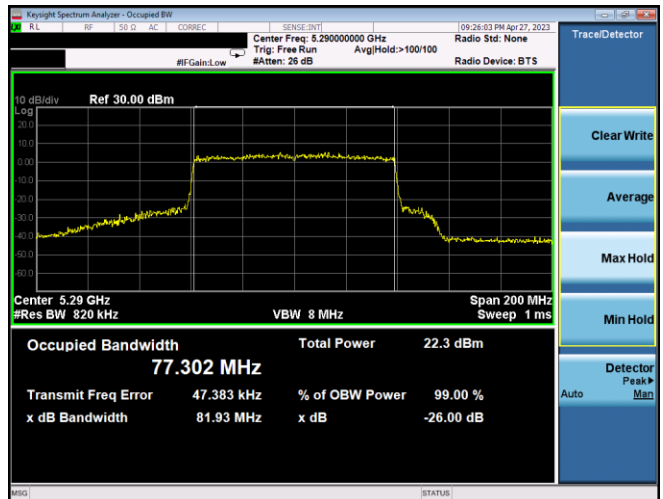
Plot 7-30. 26dB BW & 99% OBW Ant1 (80MHz BW 802.11ax(SU) – Ch. 58, MCS4)
