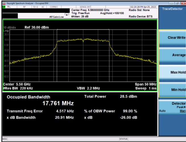
Plot 7-31. 26dB BW & 99% OBW Ant1 (20MHz BW 802.11n – Ch. 116, MCS4)
