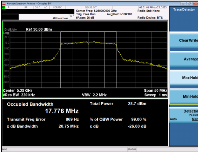
Plot 7-25. 26dB BW & 99% OBW Ant1 (20MHz BW 802.11n – Ch. 56, MCS4)
