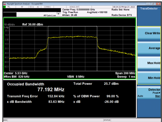
Plot 7-18. 26dB BW & 99% OBW Ant1 (80MHz BW 802.11ax(SU) – Ch. 106, MCS2)
