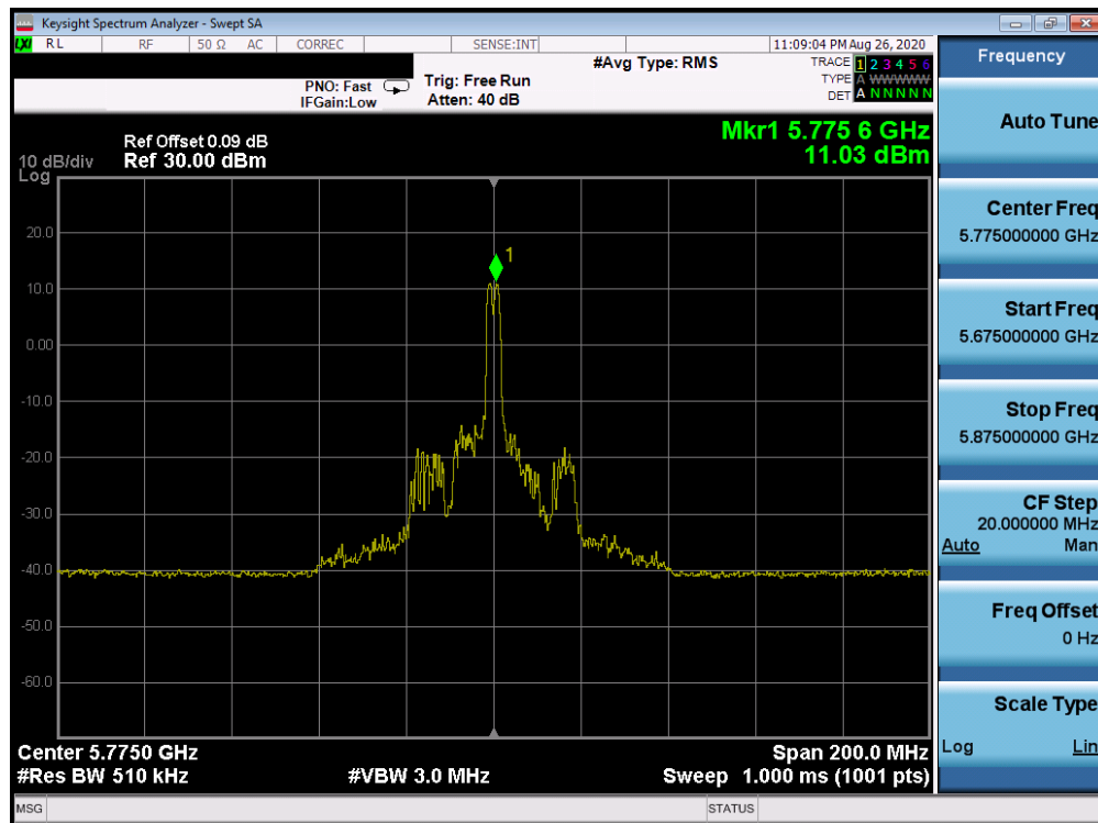
Plot 7-1170. Power Spectral Density Plot CDD Diversity Antenna 1b (80MHz BW 802.11ax Index 18 – RU26 (UNII Band 3) – Ch. 155)
