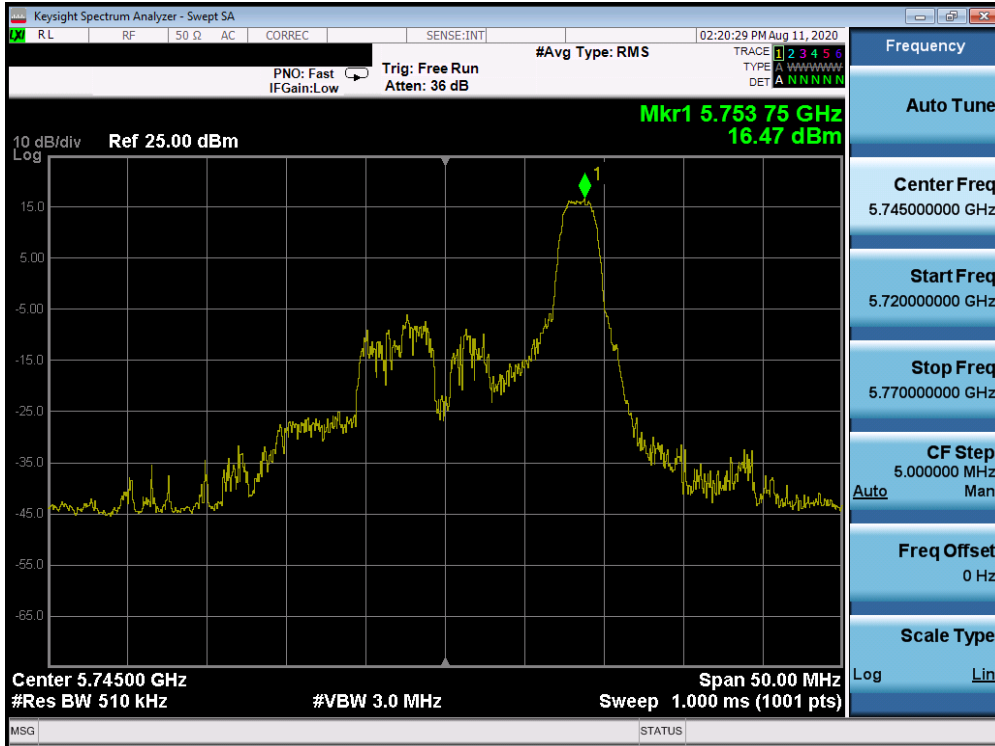
Plot 7-871. Power Spectral Density Plot CDD Primary Antenna 2b (20MHz BW 802.11ax Index 8 – RU26 (UNII Band 3) – Ch. 149)
