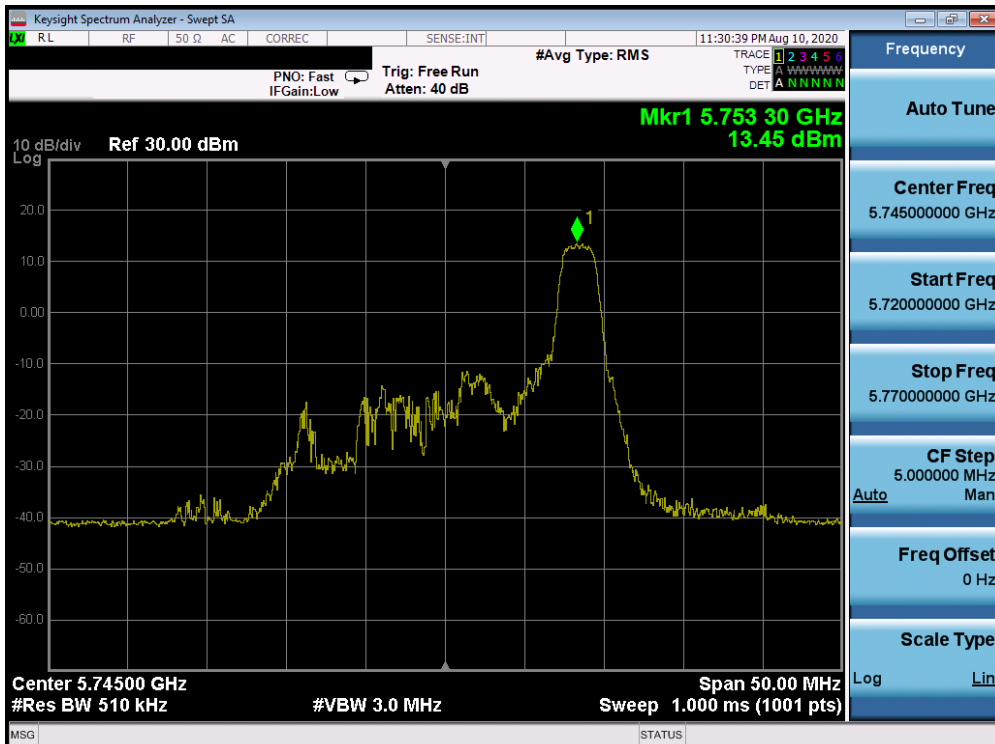
Plot 7-872. Power Spectral Density Plot CDD Primary Antenna 2a (20MHz BW 802.11ax Index 8 – RU26 (UNII Band 3) – Ch. 149)
