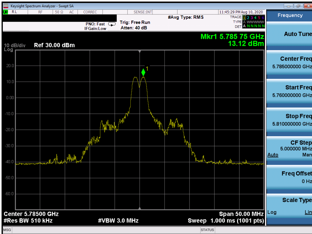
Plot 7-876. Power Spectral Density Plot CDD Primary Antenna 2a (20MHz BW 802.11ax Index 4 – RU26 (UNII Band 3) – Ch. 157)
