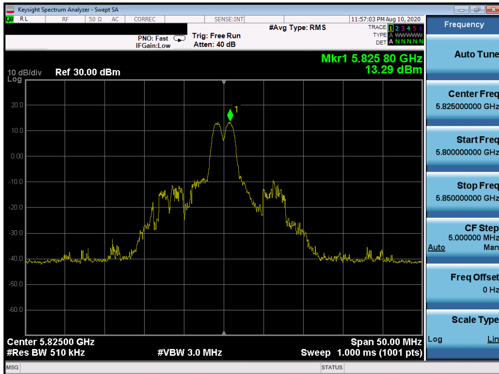
Plot 7-882. Power Spectral Density Plot CDD Primary Antenna 2a (20MHz BW 802.11ax Index 4 – RU26 (UNII Band 3) – Ch. 165)
