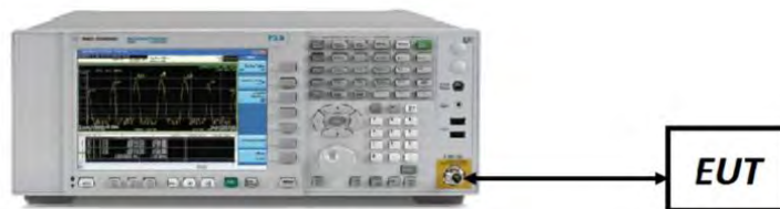
Figure 7-3. Test Instrument & Measurement Setup
