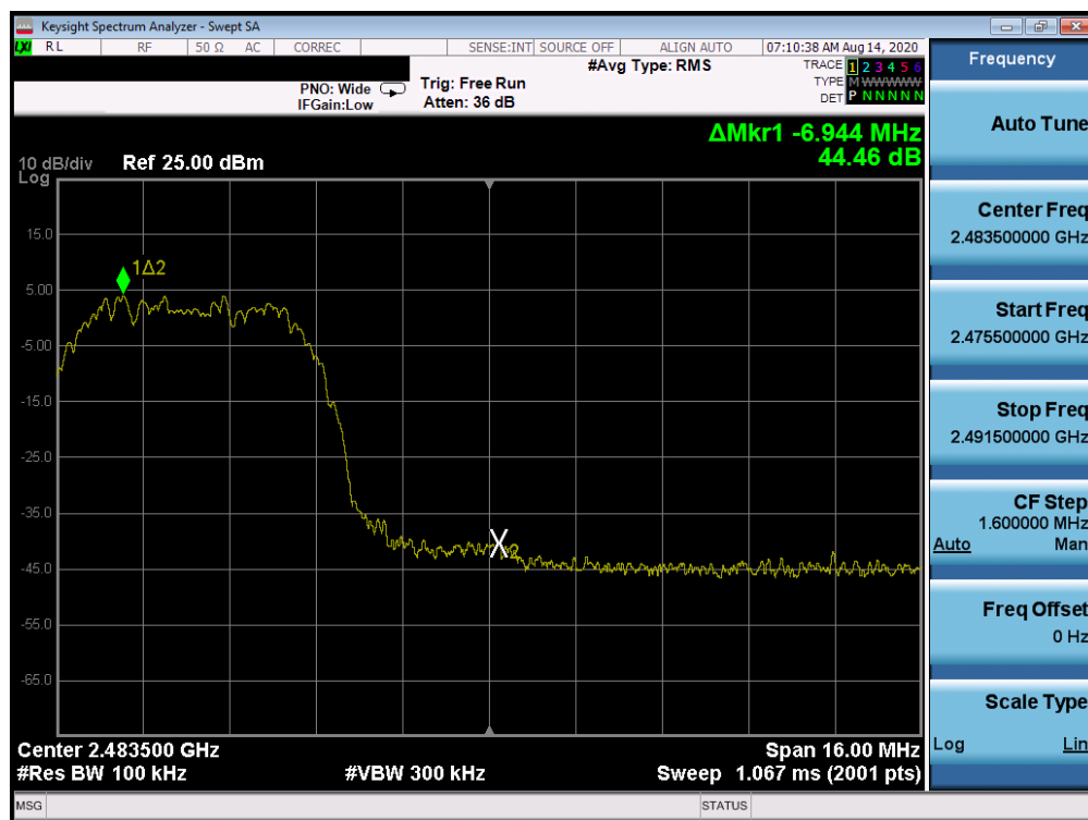
Plot 7-68. Band Edge Plot Antenna 1a (Bluetooth (HDR8), ePA - Ch. 75)
