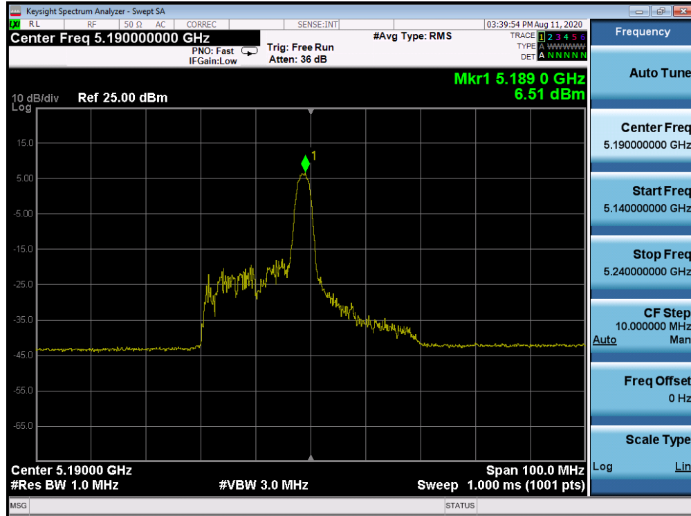
Plot 7-989. Power Spectral Density Plot CDD Diversity Antenna 2b (40MHz BW 802.11ax Index 8 – RU26 (UNII Band 1) – Ch. 38)
