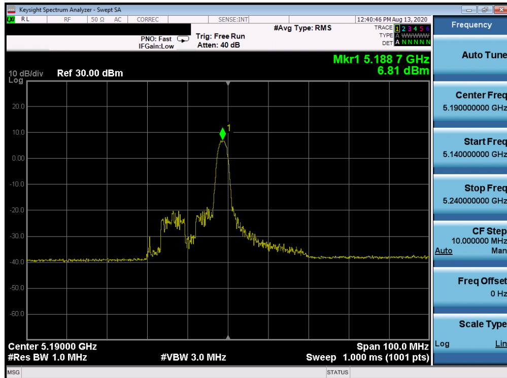
Plot 7-990. Power Spectral Density Plot CDD Diversity Antenna 1b (40MHz BW 802.11ax Index 8 – RU26 (UNII Band 1) – Ch. 38)
