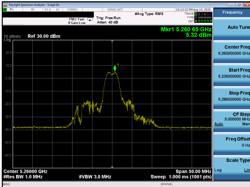
Plot 7-754. Power Spectral Density Plot CDD Primary Antenna 2a (20MHz BW 802.11ax Index 4 – RU26 (UNII Band 2A) – Ch. 52)
