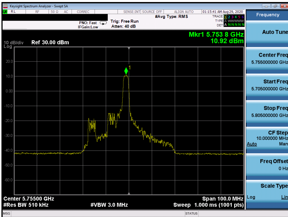
Plot 7-538. Power Spectral Density Plot Antenna 2a (40MHz BW 802.11ax Index 8 – RU26 (UNII Band 3) – Ch. 151)
