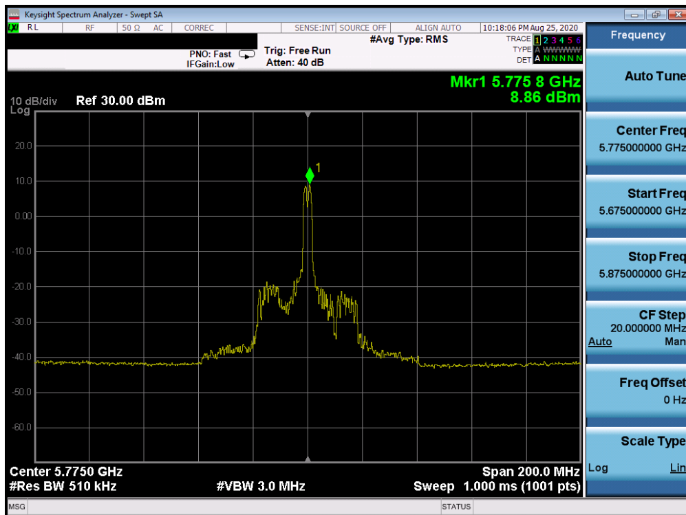
Plot 7-546. Power Spectral Density Plot Antenna 2a (80MHz BW 802.11ax Index 18 – RU26 (UNII Band 3) – Ch. 155)
