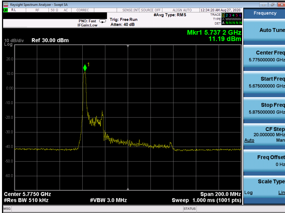
Plot 7-415. Power Spectral Density Plot Antenna 2b (80MHz BW 802.11ax Index 0 – RU26 (UNII Band 3) – Ch. 155)
