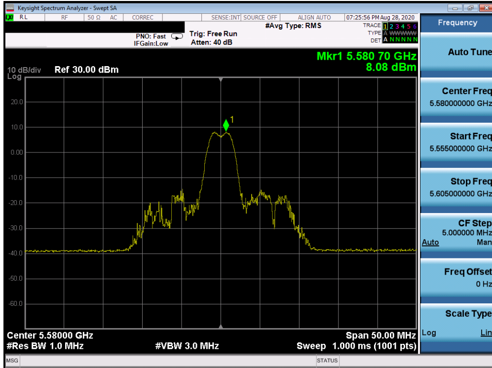
Plot 7-365. Power Spectral Density Plot Antenna 2b (20MHz BW 802.11ax Index 4 – RU26 (UNII Band 2C) – Ch. 116)
