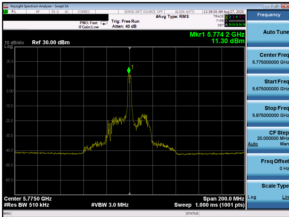
Plot 7-416. Power Spectral Density Plot Antenna 2b (80MHz BW 802.11ax Index 18 – RU26 (UNII Band 3) – Ch. 155)
