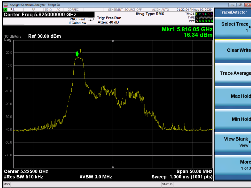
Plot 7-401. Power Spectral Density Plot Antenna 2b (20MHz BW 802.11ax Index 0 – RU26 (UNII Band 3) – Ch. 165)
