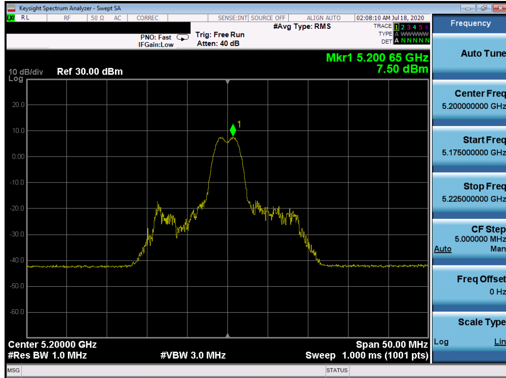
Plot 7-317. Power Spectral Density Plot Antenna 2b (20MHz BW 802.11ax Index 4 – RU26 (UNII Band 1) – Ch. 40)
