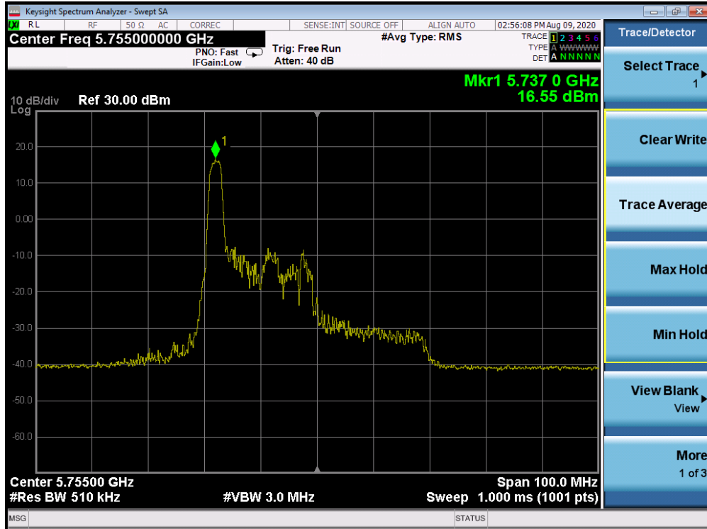
Plot 7-407. Power Spectral Density Plot Antenna 2b (40MHz BW 802.11ax Index 0 – RU26 (UNII Band 3) – Ch. 151)
