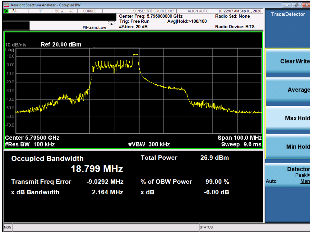
Plot 7-281. 6dB Bandwidth Plot Antenna 2a (40MHz BW 802.11ax Index 8 – RU26 (UNII Band 3) – Ch. 159)
