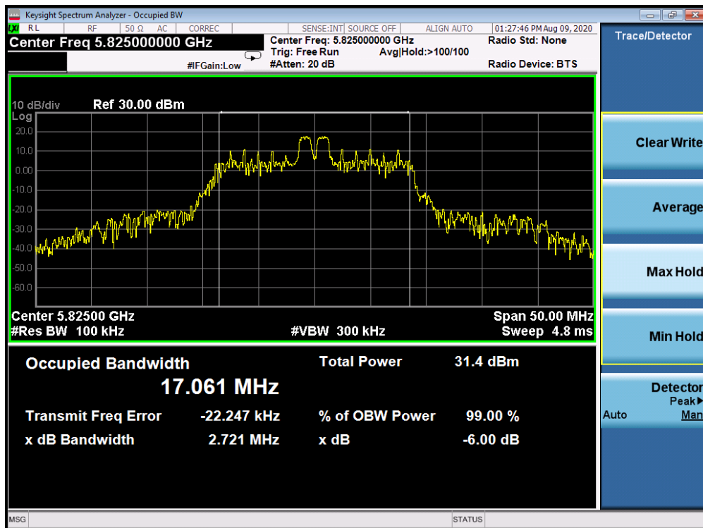
Plot 7-248. 6dB Bandwidth Plot Antenna 2b (20MHz BW 802.11ax Index 4 – RU26 (UNII Band 3) – Ch. 165)
