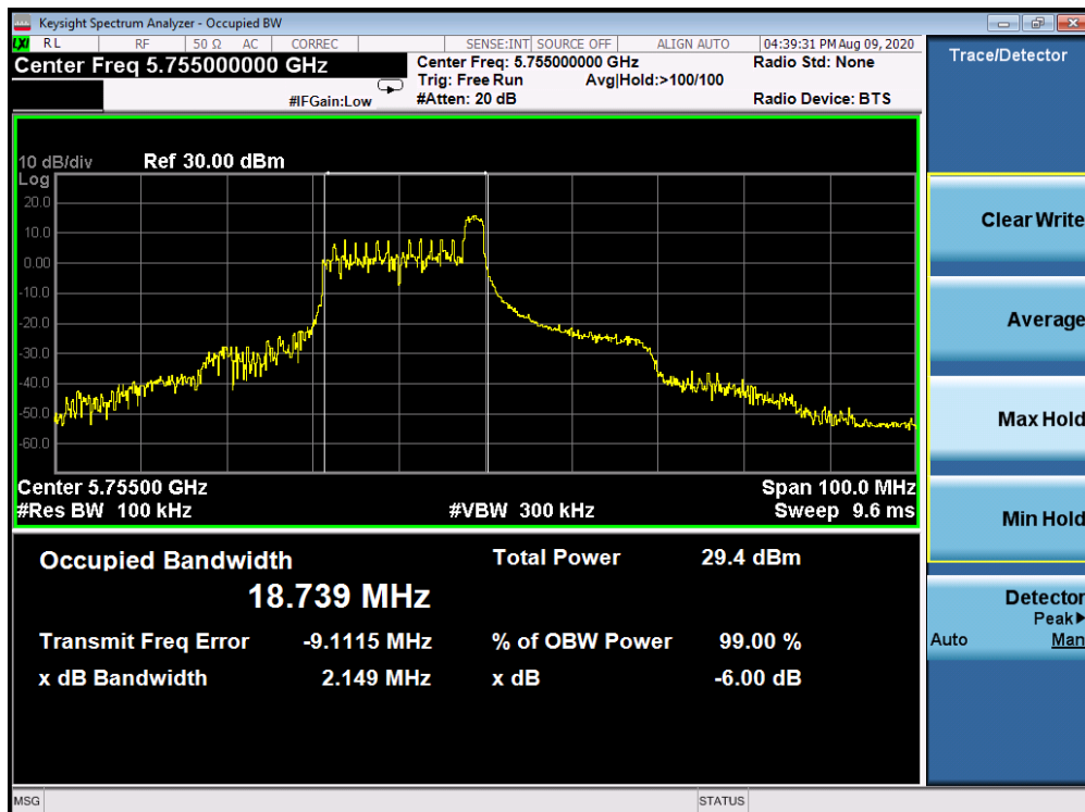
Plot 7-302. 6dB Bandwidth Plot Antenna 1b (40MHz BW 802.11ax Index 8 – RU26 (UNII Band 3) – Ch. 151)
