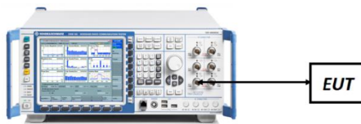
Figure 7-7. ERP/EIRP Measurement Setup
