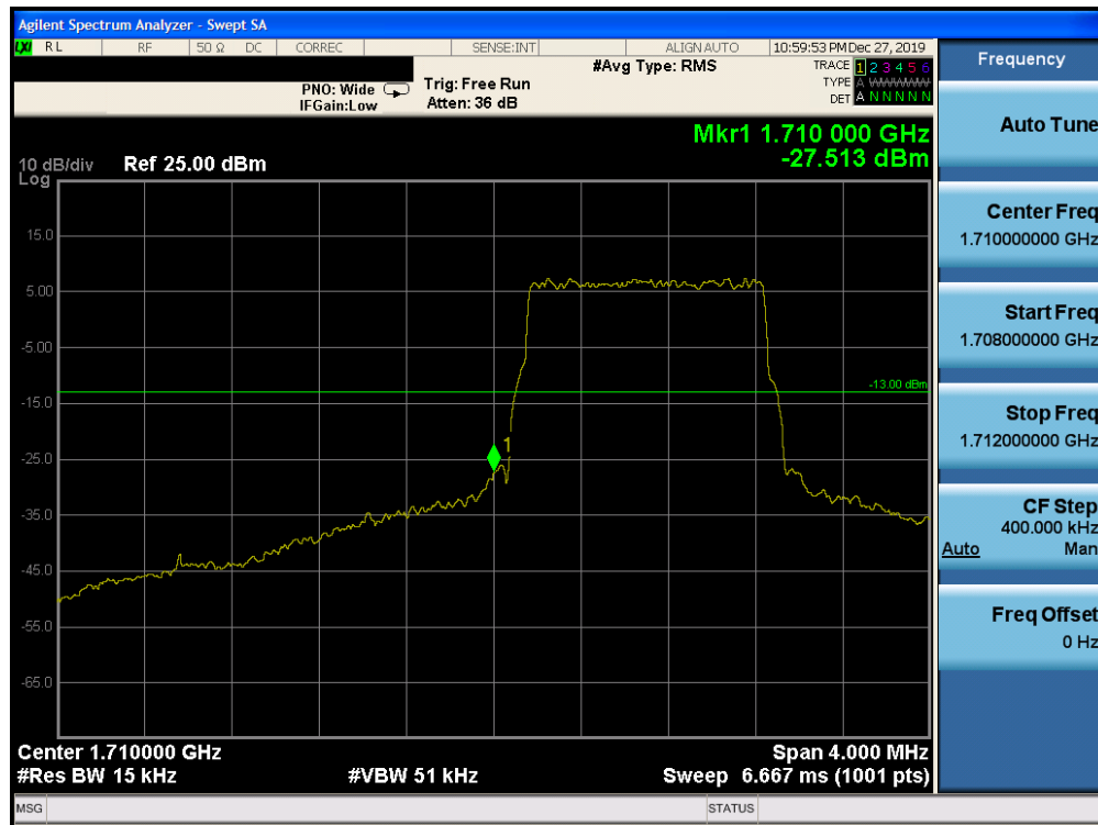
Plot 7-234. Lower Band Edge Plot (Band 4 – 1.4MHz QPSK – RB Size 6)
