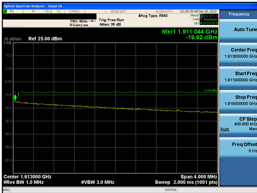
Plot 7-297. Upper Extended Band Edge Plot (Band 2 – 10.0MHz QPSK – RB Size 50)
