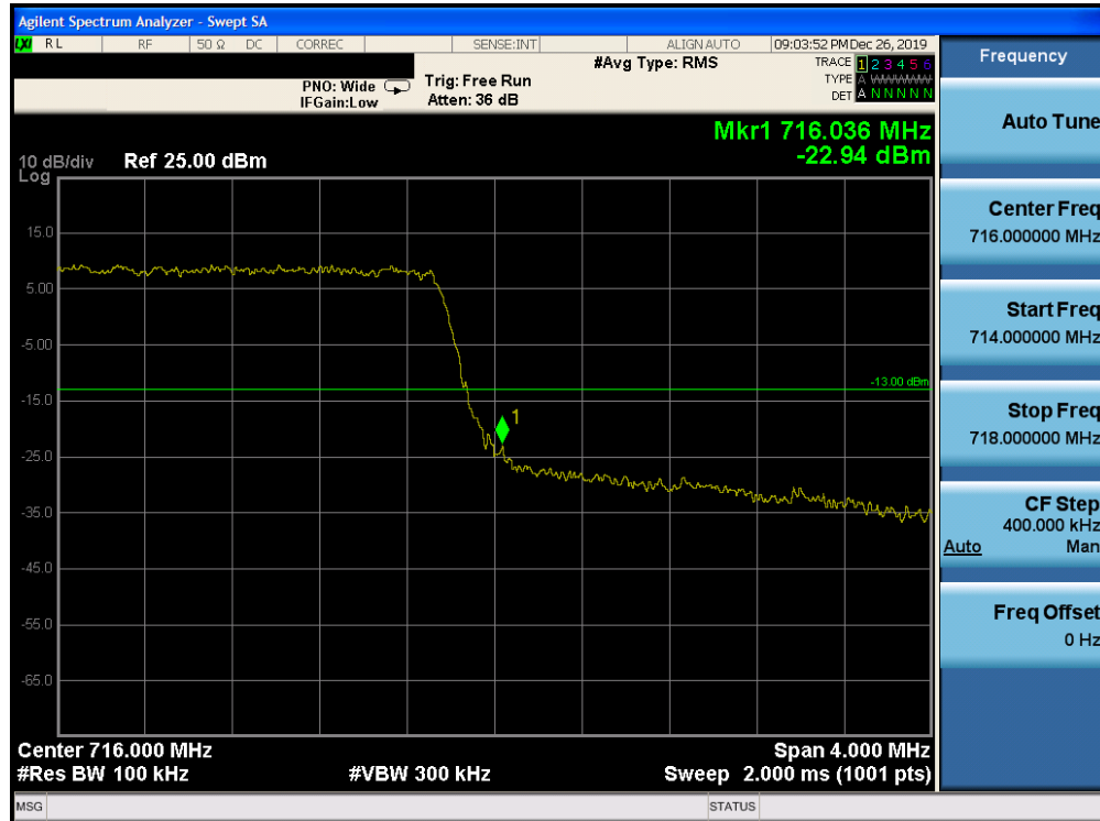
Plot 7-207. Upper Band Edge Plot (Band 17 – 5.0MHz QPSK – RB Size 25)
