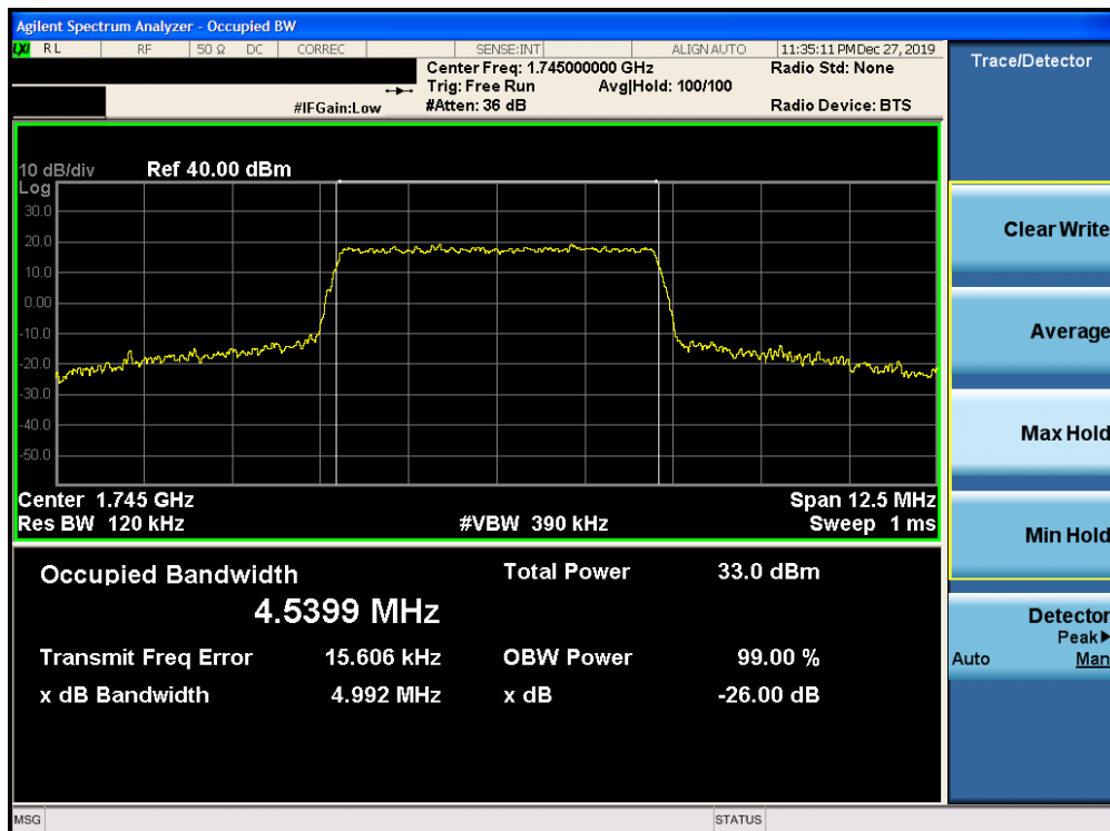
Plot 7-50. Occupied Bandwidth Plot (Band 66/4 – 5.0MHz 16-QAM – RB Size 25)
