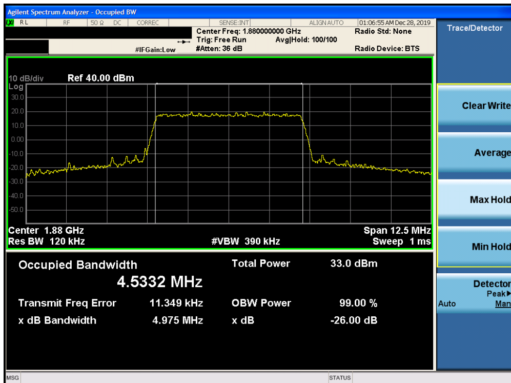
Plot 7-68. Occupied Bandwidth Plot (Band 25/2 – 5.0MHz 16-QAM – RB Size 25)
