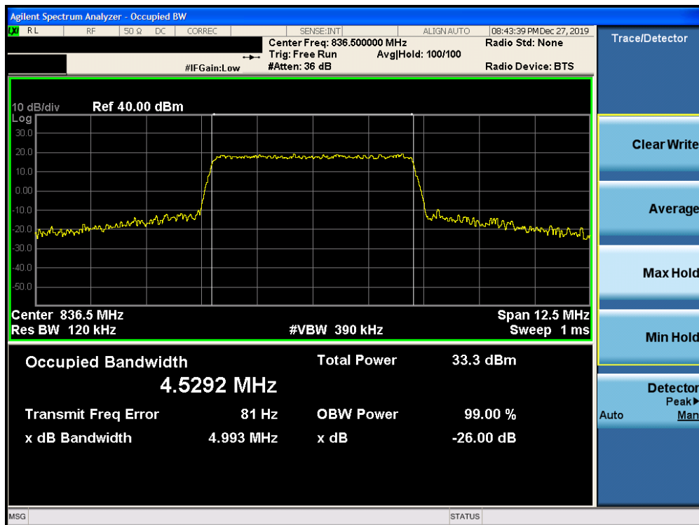
Plot 7-38. Occupied Bandwidth Plot (Band 26/5 – 5.0MHz 16-QAM – RB Size 25)
