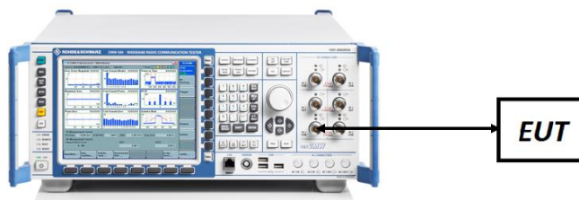
Figure 7-5. ERP/EIRP Measurement Setup
