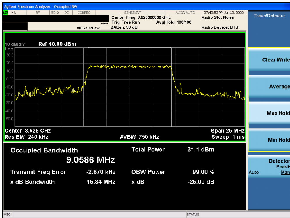
Plot 7-8. Occupied Bandwidth Plot (LTE Band 48 - 10MHz 16-QAM - Full RB Configuration)
