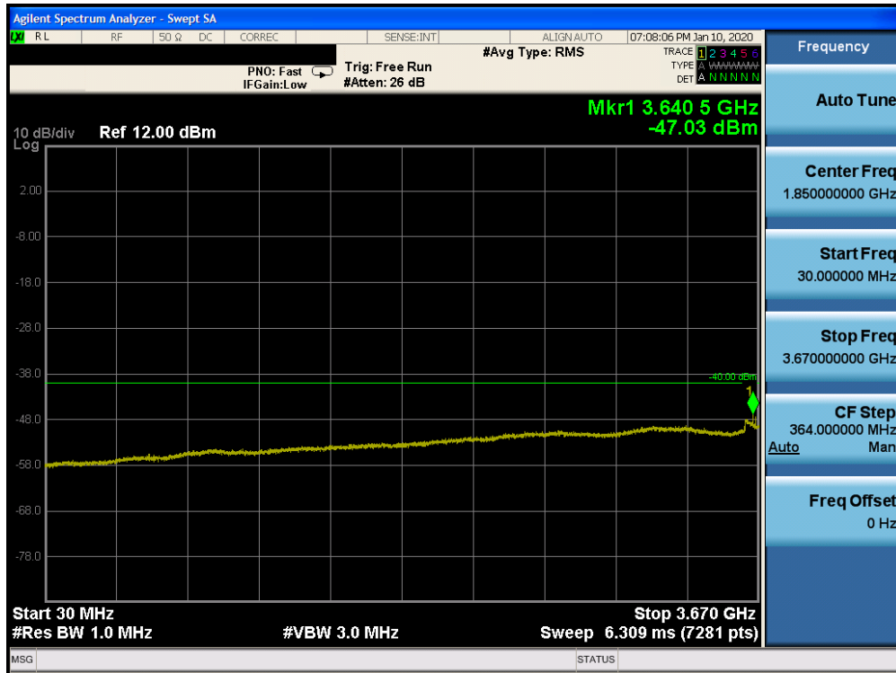
Plot 7-21. Conducted Spurious Plot (LTE Band 48 - 20MHz QPSK - RB Size 1, RB Offset 0 - High Channel)
