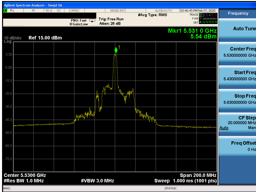
Plot 7-611. Power Spectral Density Plot SDM CORE 0 (80MHz BW 802.11ax Index 18 – RU26 (UNII Band 2C) – Ch. 106)
