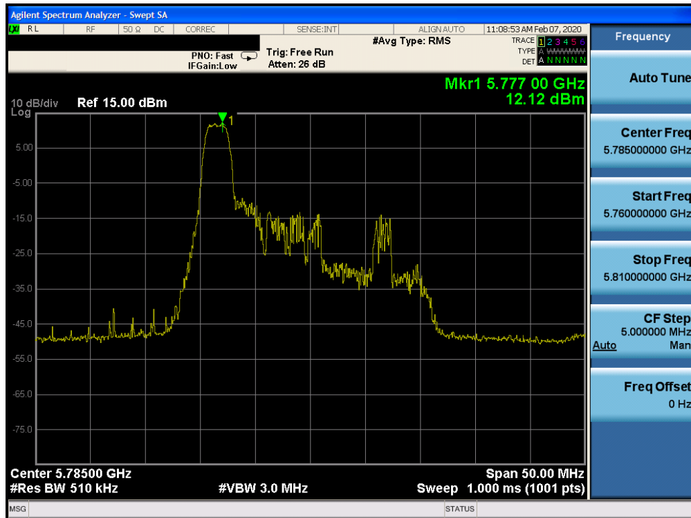
Plot 7-679. Power Spectral Density Plot CDD CORE 0 (20MHz BW 802.11ax Index 0 – RU26 (UNII Band 3) – Ch. 157)
