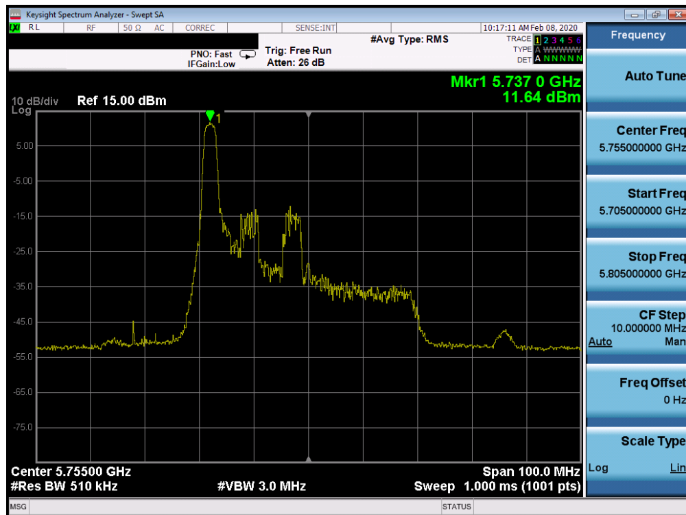
Plot 7-698. Power Spectral Density Plot CDD CORE 1 (40MHz BW 802.11ax Index 0 – RU26 (UNII Band 3) – Ch. 151)
