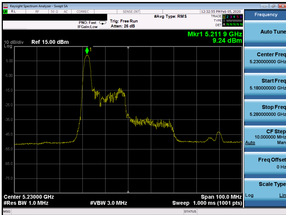
Plot 7-352. Power Spectral Density Plot SISO CORE 1 (40MHz BW 802.11ax Index 0 – RU26 (UNII Band 1) – Ch. 46)
