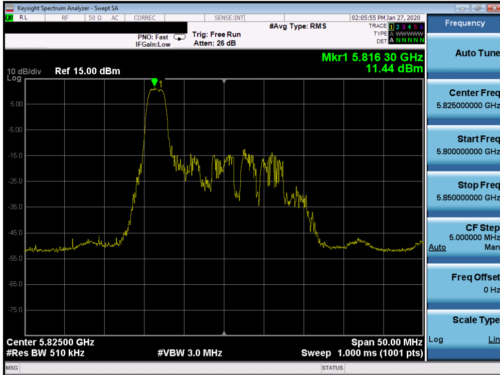
Plot 7-447. Power Spectral Density Plot SISO CORE 1 (20MHz BW 802.11ax Index 0 – RU26 (UNII Band 3) – Ch. 165)
