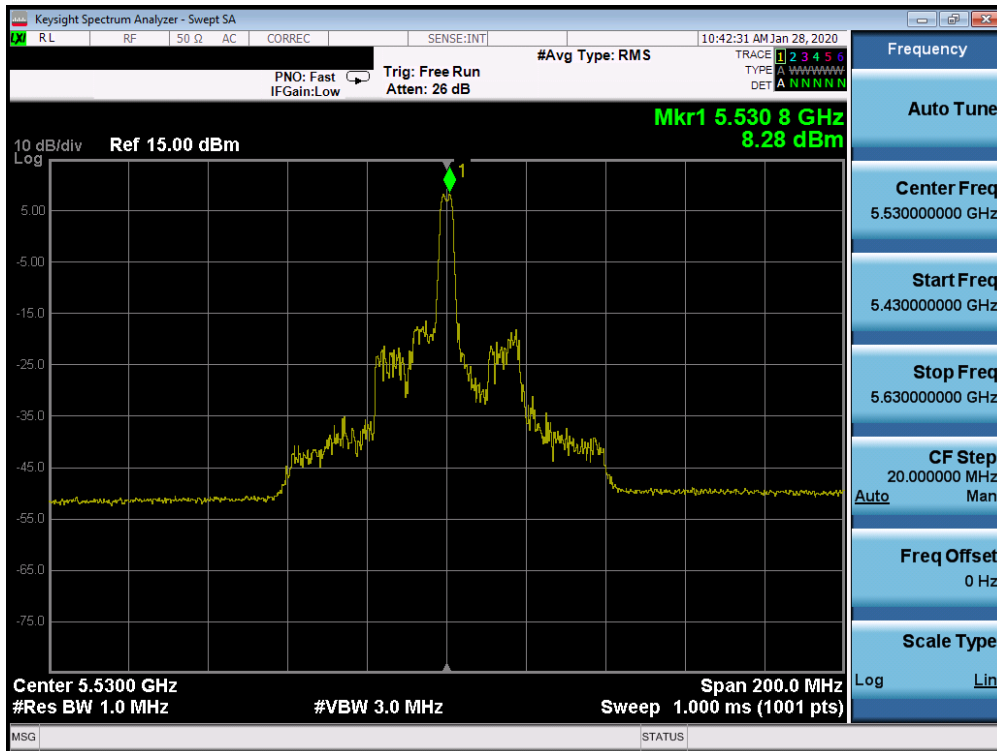
Plot 7-410. Power Spectral Density Plot SISO CORE 1 (80MHz BW 802.11ax Index 18 – RU26 (UNII Band 2C) – Ch. 106)
