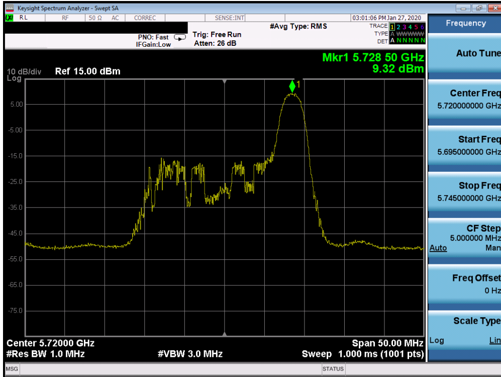
Plot 7-393. Power Spectral Density Plot SISO CORE 1 (20MHz BW 802.11ax Index 8 – RU26 (UNII Band 2C) – Ch. 144)
