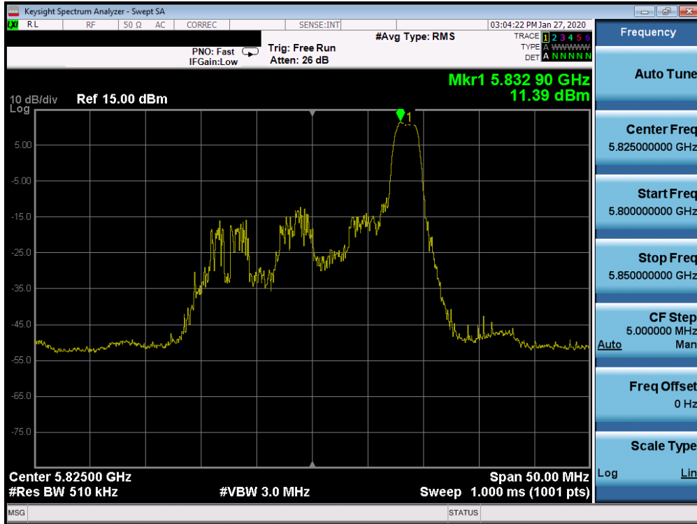
Plot 7-449. Power Spectral Density Plot SISO CORE 1 (20MHz BW 802.11ax Index 8 – RU26 (UNII Band 3) – Ch. 165)
