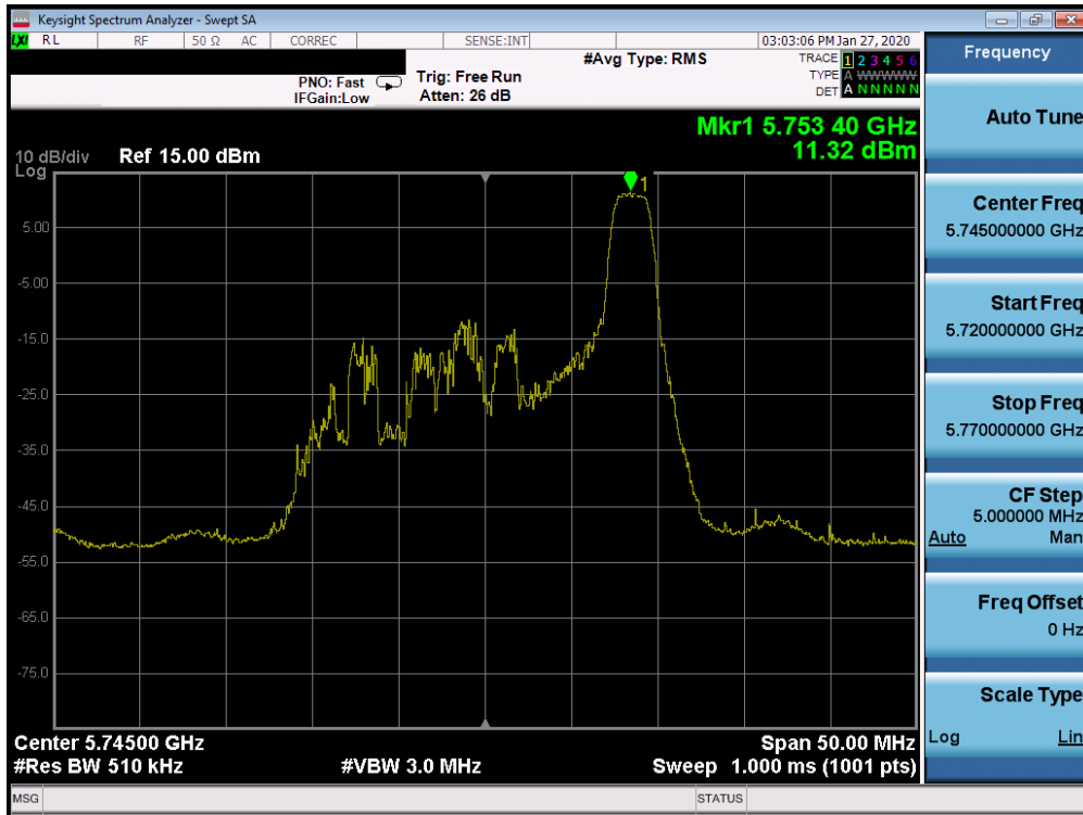
Plot 7-443. Power Spectral Density Plot SISO CORE 1 (20MHz BW 802.11ax Index 8 – RU26 (UNII Band 3) – Ch. 149)
