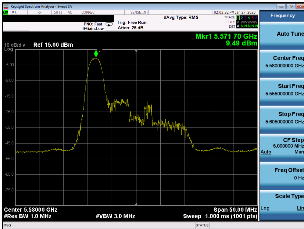
Plot 7-388. Power Spectral Density Plot SISO CORE 1 (20MHz BW 802.11ax Index 0 – RU26 (UNII Band 2C) – Ch. 116)
