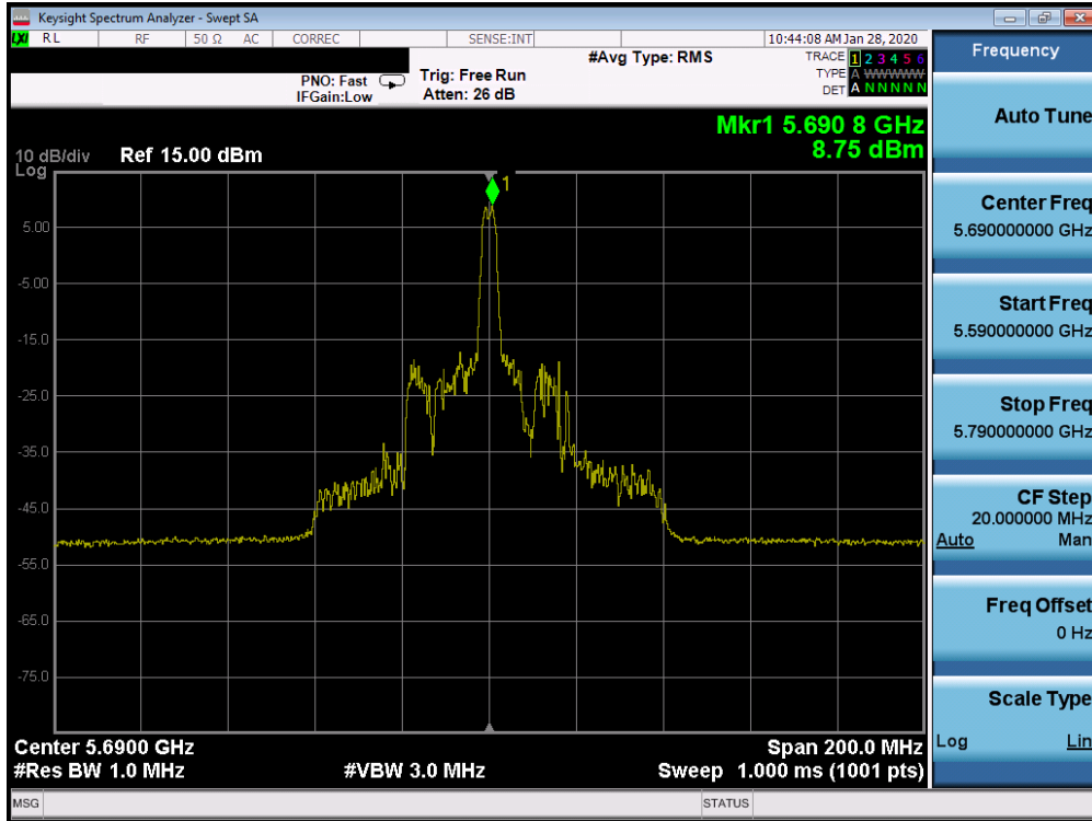
Plot 7-413. Power Spectral Density Plot SISO CORE 1 (80MHz BW 802.11ax Index 18 – RU26 (UNII Band 2C) – Ch. 138)
