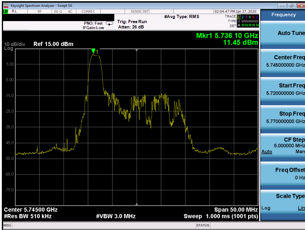
Plot 7-441. Power Spectral Density Plot SISO CORE 1 (20MHz BW 802.11ax Index 0 – RU26 (UNII Band 3) – Ch. 149)
