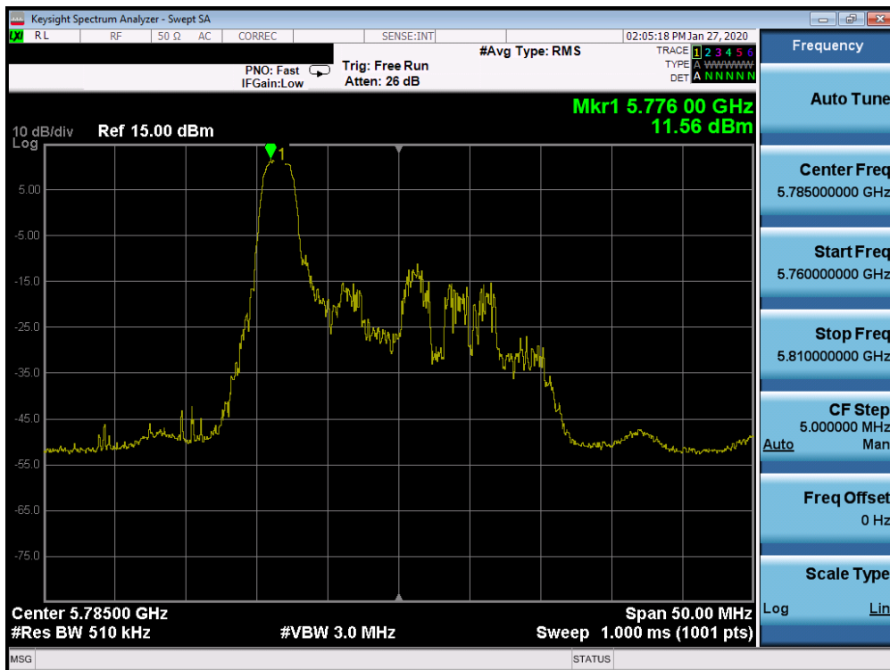
Plot 7-444. Power Spectral Density Plot SISO CORE 1 (20MHz BW 802.11ax Index 0 – RU26 (UNII Band 3) – Ch. 157)
