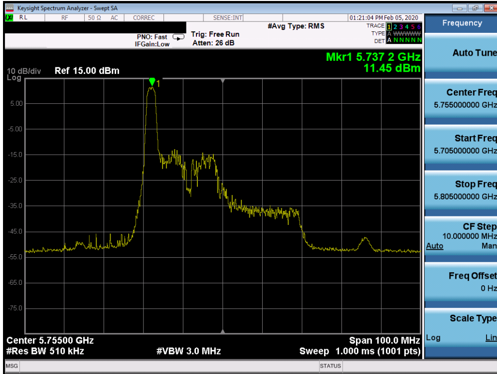
Plot 7-453. Power Spectral Density Plot SISO CORE 1 (40MHz BW 802.11ax Index 0 – RU26 (UNII Band 3) – Ch. 151)
