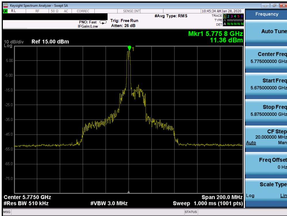
Plot 7-462. Power Spectral Density Plot SISO CORE 1 (80MHz BW 802.11ax Index 18 – RU26 (UNII Band 3) – Ch. 155)
