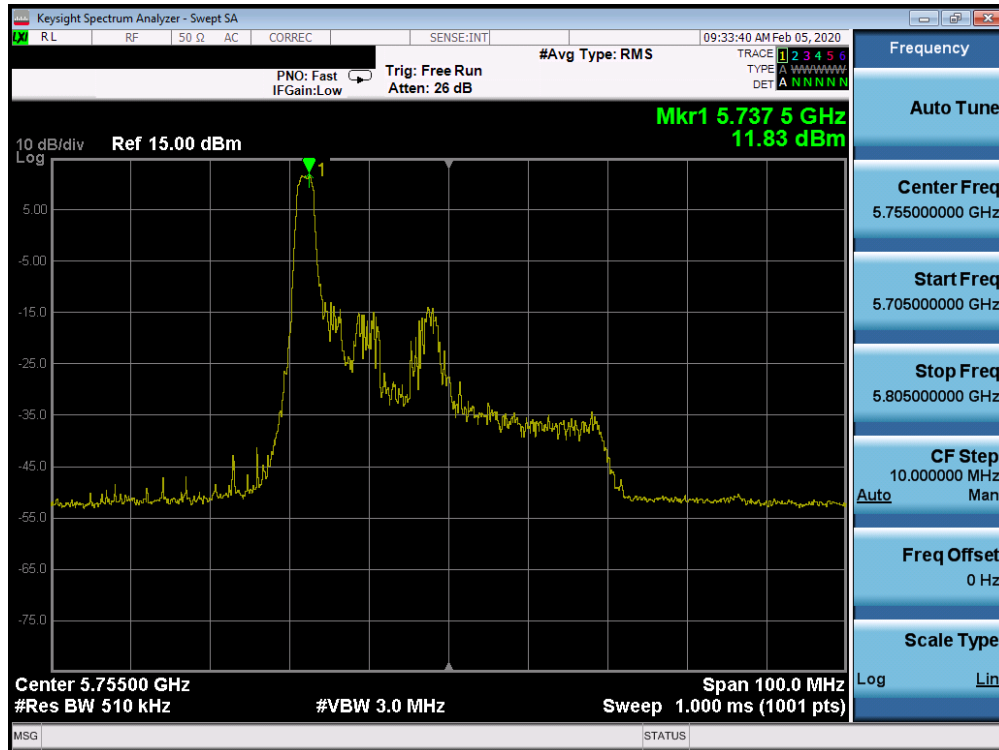
Plot 7-325. Power Spectral Density Plot SISO CORE 0 (40MHz BW 802.11ax Index 0 – RU26 (UNII Band 3) – Ch. 151)
