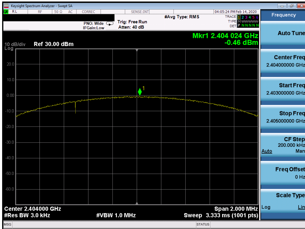
Plot 7-49. Power Spectral Density Plot Tx BF Ant 4a (Bluetooth (LE), 2Mbps, ePA – Ch. 1)
