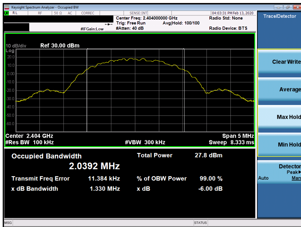
Plot 7-4. 6dB Bandwidth Plot Ant 4a (Bluetooth (LE), 2Mbps, ePA – Ch. 1)
