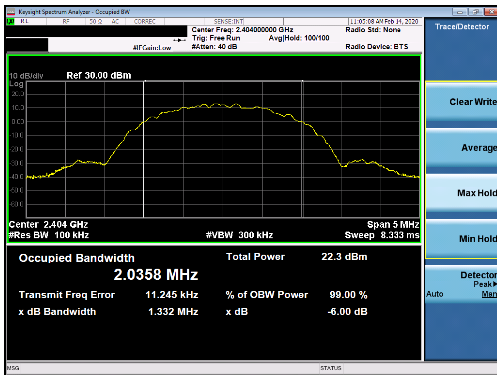
Plot 7-10. 6dB Bandwidth Plot Ant 2a (Bluetooth (LE), 2Mbps, ePA – Ch. 0)
