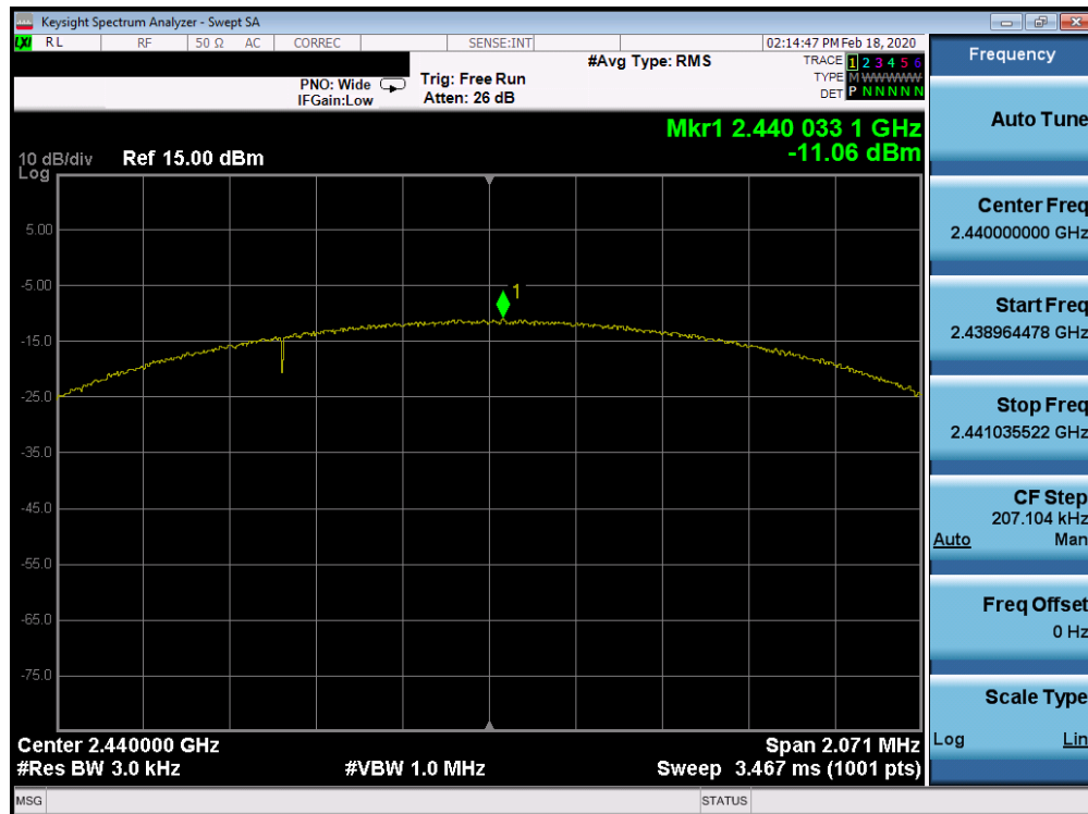
Plot 7-58. Power Spectral Density Plot TxBF Ant 2a (Bluetooth (LE), 2Mbps, iPA – Ch. 19)
