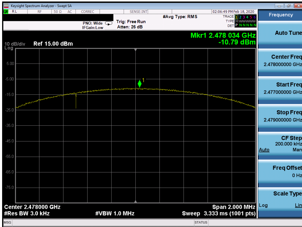
Plot 7-59. Power Spectral Density Plot TxBF Ant 4a (Bluetooth (LE), 2Mbps, iPA – Ch. 38)
