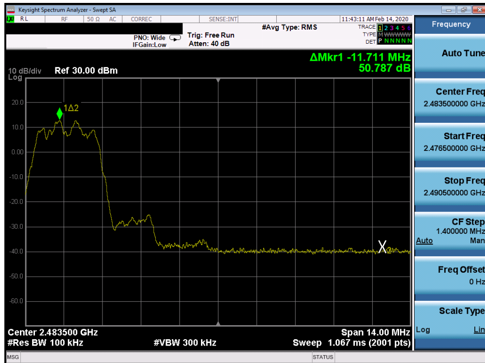
Plot 7-66. Band Edge Plot Ant 2a (Bluetooth (HDR4), ePA – Ch. 75)
