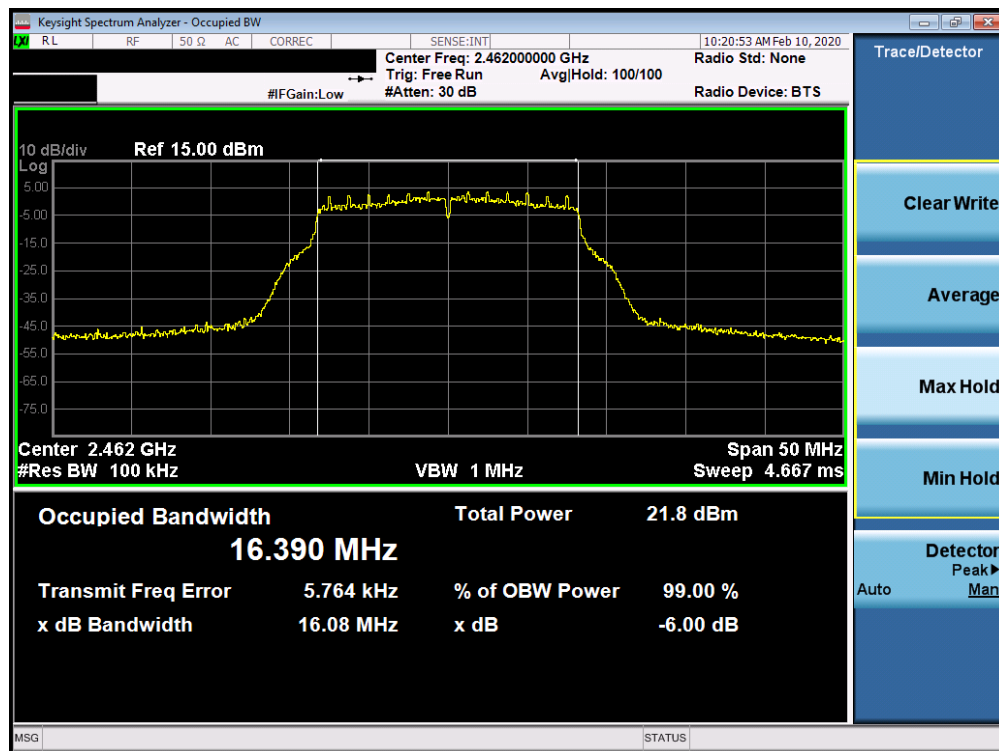
Plot 7-6. 6dB Bandwidth Plot SISO CORE0 (802.11g – Ch. 11)
