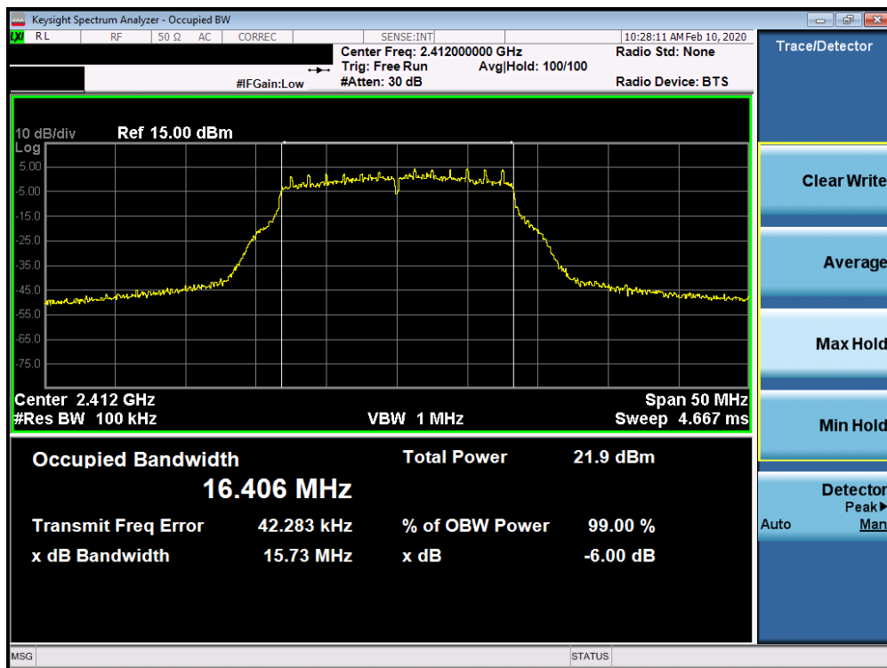
Plot 7-4. 6dB Bandwidth Plot SISO CORE0 (802.11g – Ch. 1)
