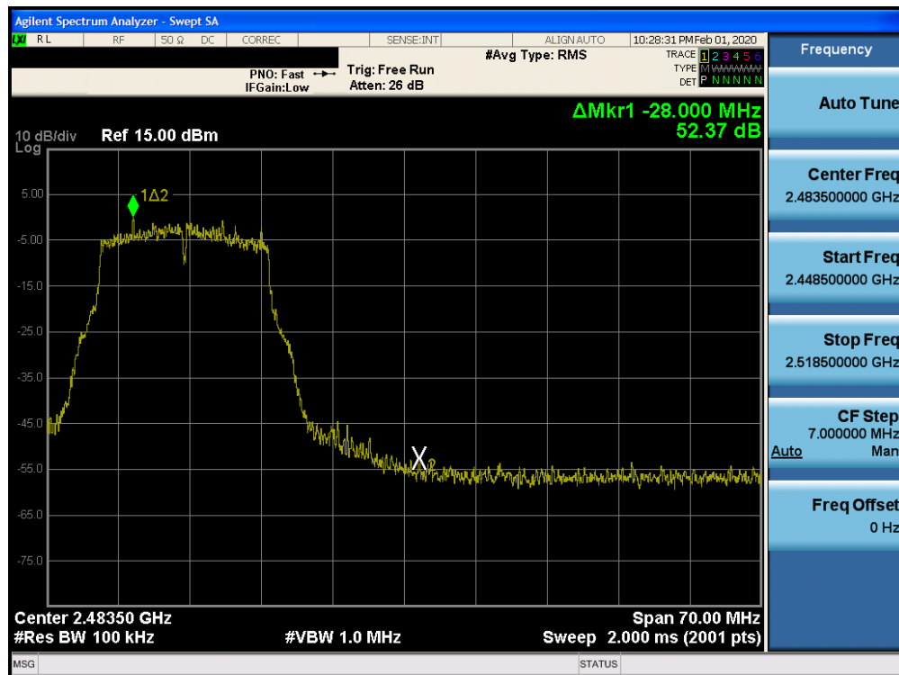
Plot 7-65. Band Edge Plot SISO CORE 1 (802.11g - Ch. 11)
