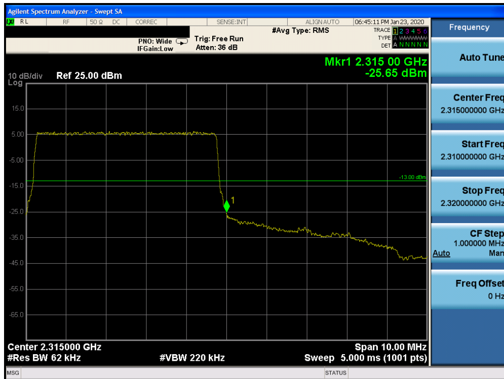
Plot 7-332. Upper Band Edge Plot (Band 30 – 5.0MHz QPSK – RB Size 25)
