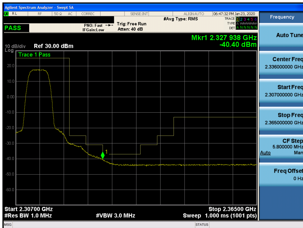
Plot 7-333. Upper Extended Band Edge Plot (Band 30 – 5.0MHz QPSK – RB Size 25)
