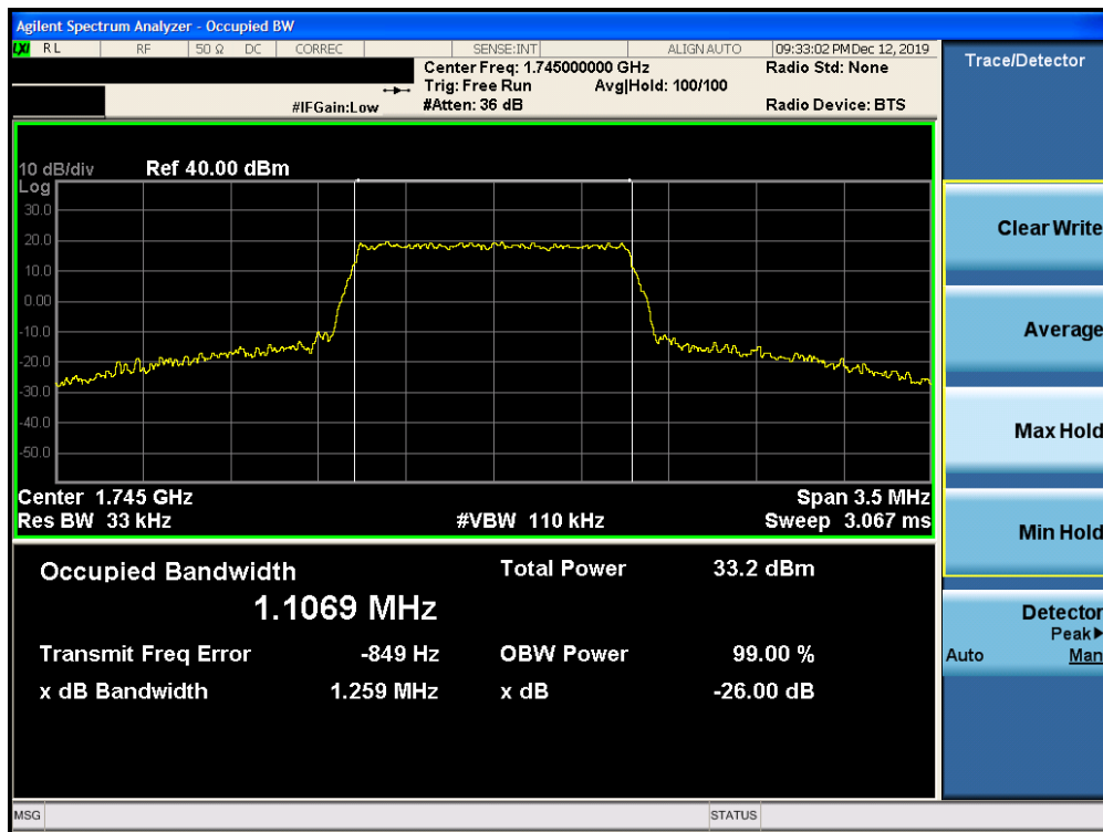
Plot 7-44. Occupied Bandwidth Plot (Band 66/4 – 1.4MHz 16-QAM – RB Size 6)
