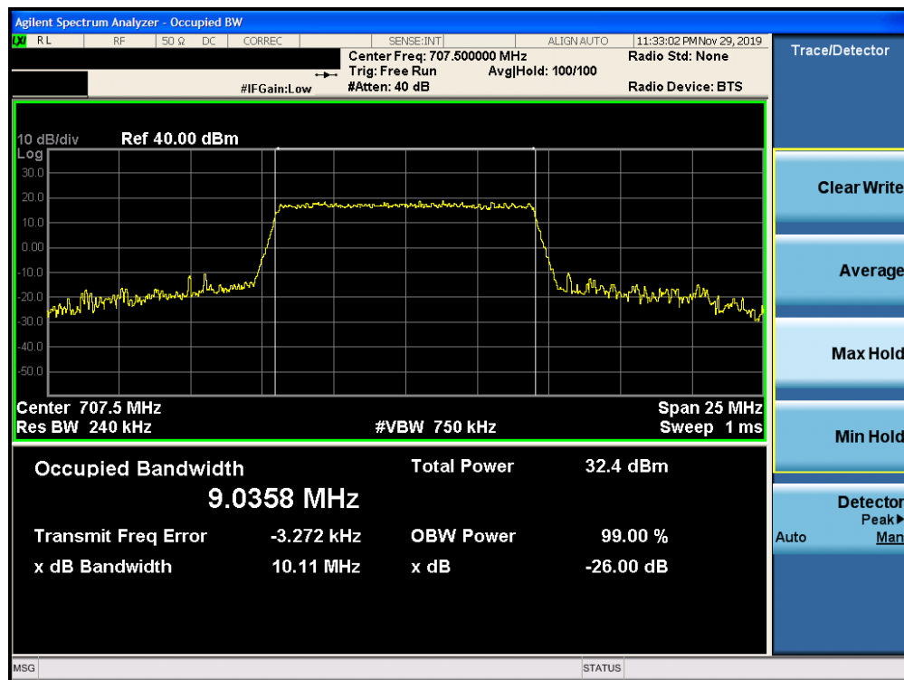
Plot 7-24. Occupied Bandwidth Plot (Band 12/17 – 10.0MHz 64-QAM – RB Size 50)
