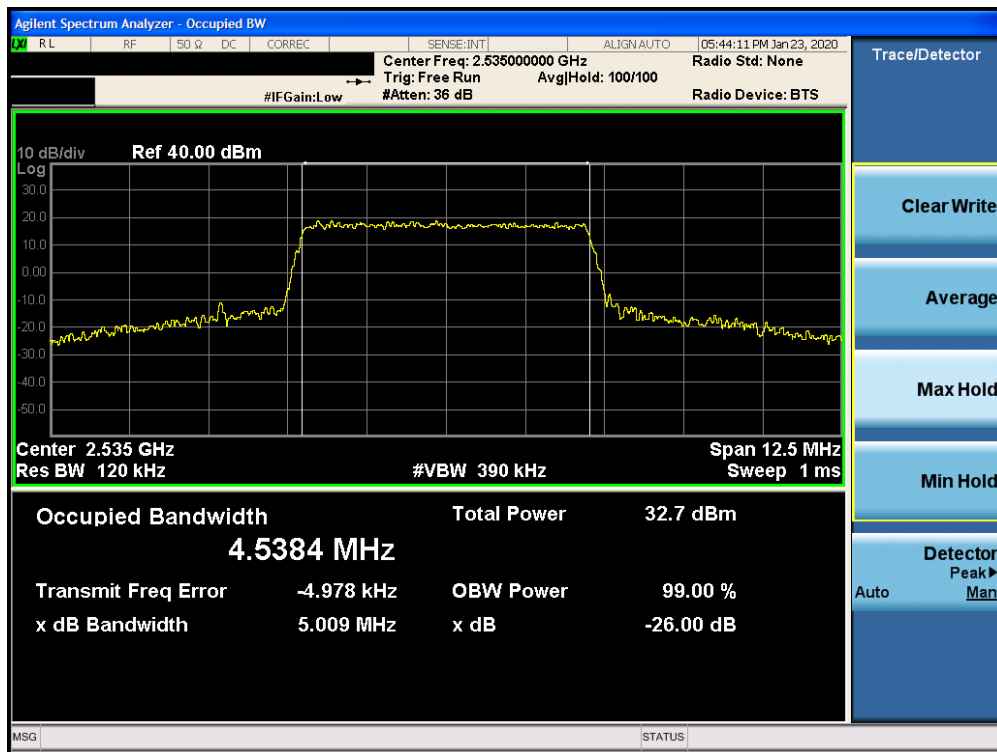
Plot 7-86. Occupied Bandwidth Plot (Band 7 – 5.0MHz 16-QAM – RB Size 25)
