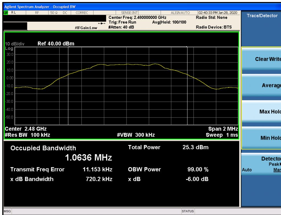
Plot 7-9. 6dB Bandwidth Plot Ant 2a (Bluetooth (LE), 1Mbps, ePA – Ch. 39)
