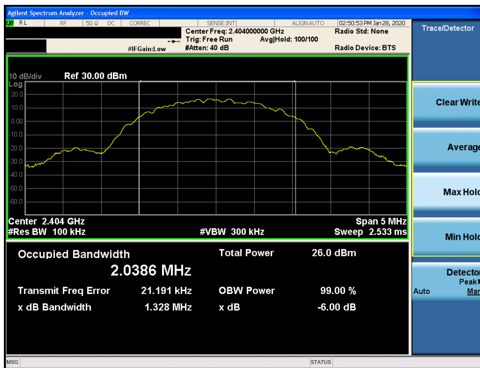
Plot 7-10. 6dB Bandwidth Plot Ant 2a (Bluetooth (LE), 2Mbps, ePA – Ch. 0)
