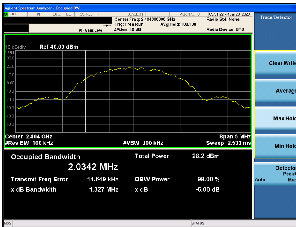
Plot 7-4. 6dB Bandwidth Plot Ant 4a (Bluetooth (LE), 2Mbps, ePA – Ch. 1)
