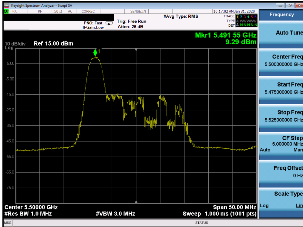
Plot 7-385. Power Spectral Density Plot SISO CORE 1 (20MHz BW 802.11ax Index 0 – RU26 (UNII Band 2C) – Ch. 100)
