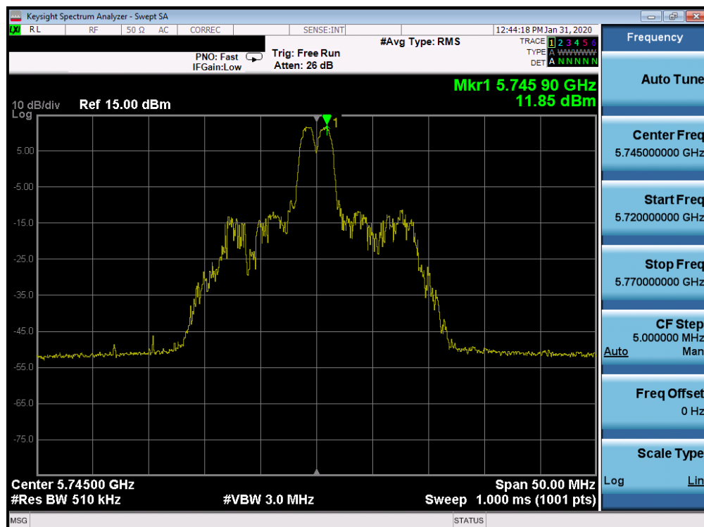
Plot 7-314. Power Spectral Density Plot SISO CORE 0 (20MHz BW 802.11ax Index 4 – RU26 (UNII Band 3) – Ch. 149)
