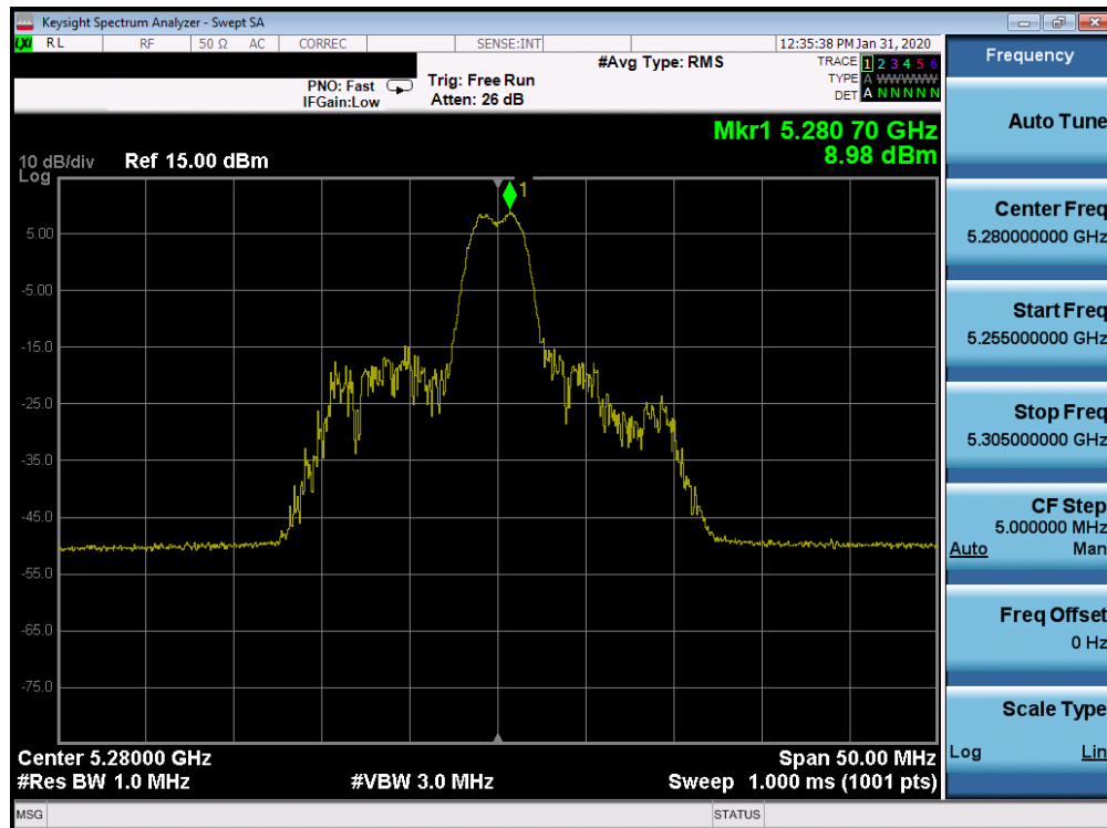
Plot 7-237. Power Spectral Density Plot SISO CORE 0 (20MHz BW 802.11ax Index 4 – RU26 (UNII Band 2A) – Ch. 56)
