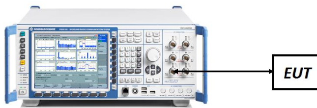
Figure 7-4. Conducted Power Measurement Setup
