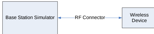
Figure 8-2 Power Measurement Setup
