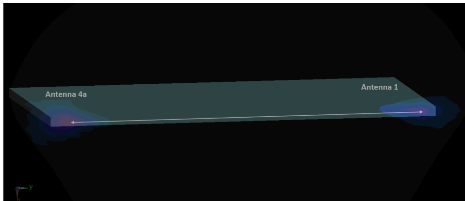
Figure 11-18 Right Edge Spatial Separation for Antenna 4A and Antenna 1
