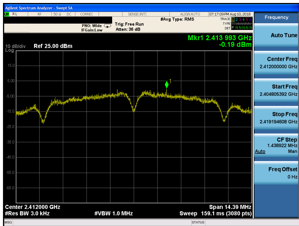
Plot 7-46. Power Spectral Density Plot SISO CORE1 DIVERSITY (802.11b - Ch. 1)
