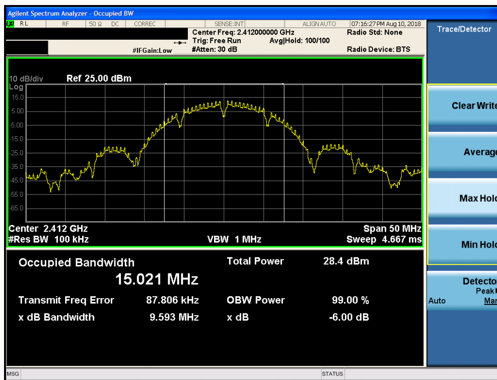
Plot 7-19. 6dB Bandwidth Plot SISO CORE1 DIVERSITY (802.11b – Ch. 1)
