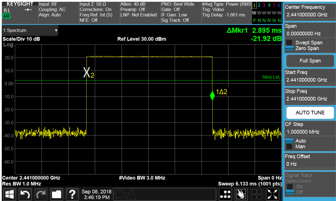
Plot 7-49. Time of Occupancy Plot ANT0(Bluetooth, GFSK, ePA)
