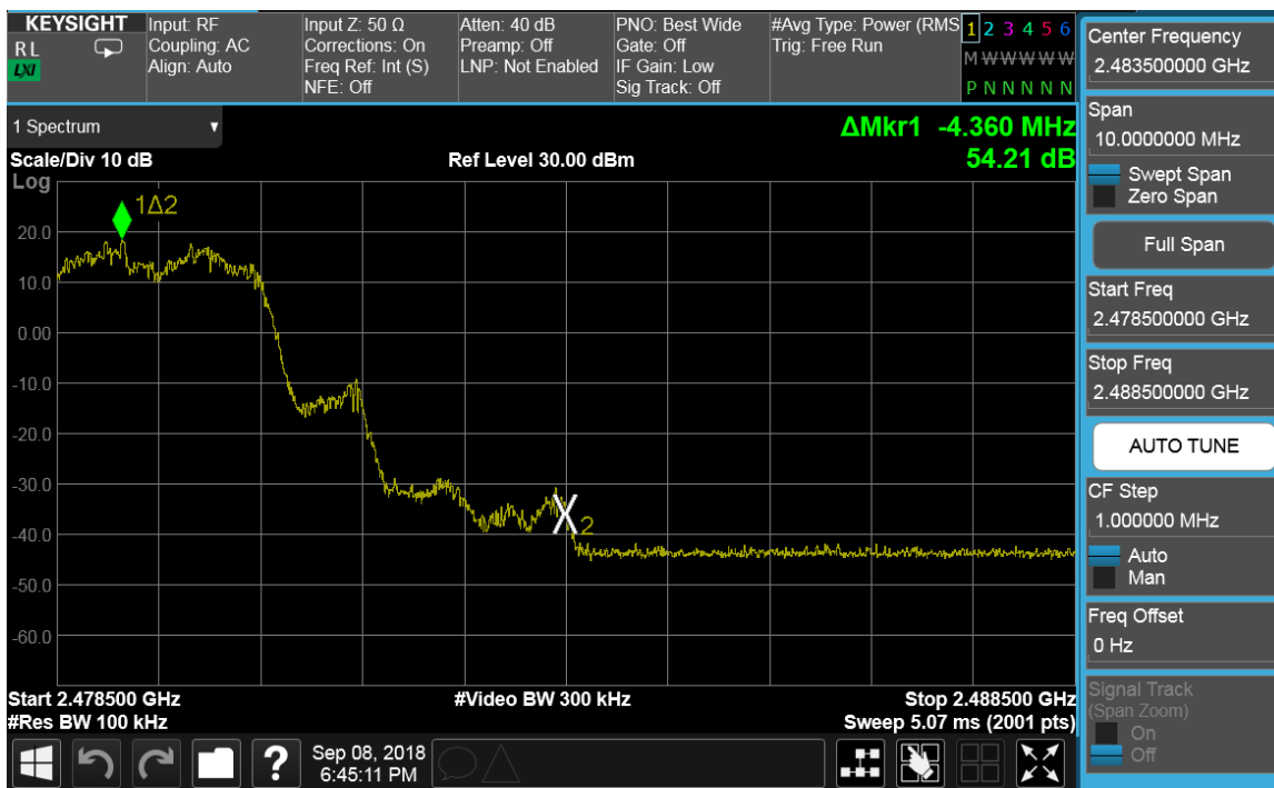
Plot 7-26. Band Edge Plot ANT 0 (Bluetooth with Hopping Enabled, 8DPSK, ePA)
