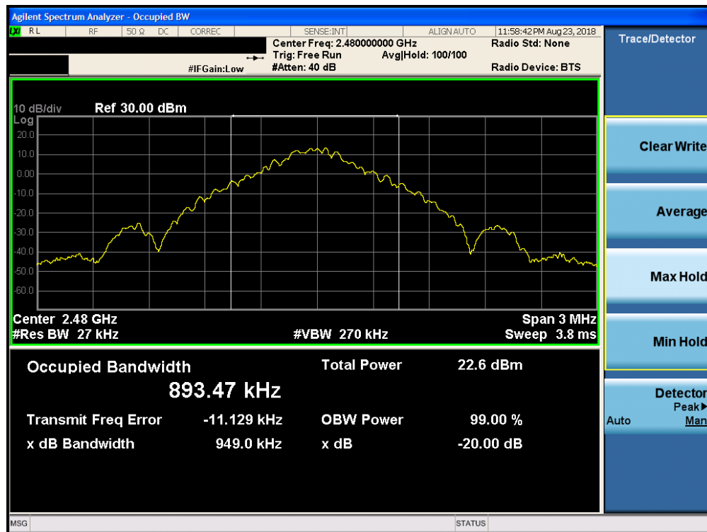
Plot 7-15. 20dB Bandwidth Plot ANT 2 (Bluetooth, GFSK, ePA – Ch. 78)
