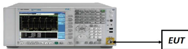
Figure 7-3. Test Instrument & Measurement Setup
