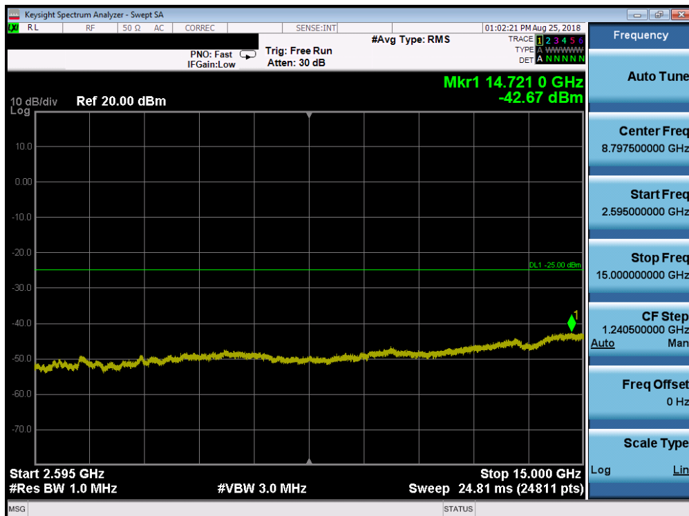
Plot 7-173. Conducted Spurious Plot (Band 7 – 20.0MHz QPSK – RB Size 1, RB Offset 0 – High Channel)
