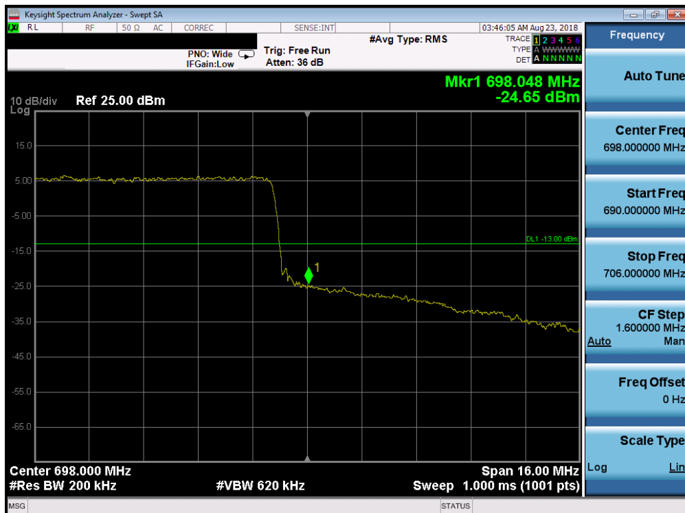
Plot 7-191. Upper Band Edge Plot (Band 71 – 20.0MHz QPSK – RB Size 100)
