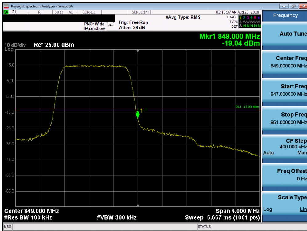
Plot 7-213. Upper Band Edge Plot (Band 5 - 1.4MHz QPSK - RB Size 6)
