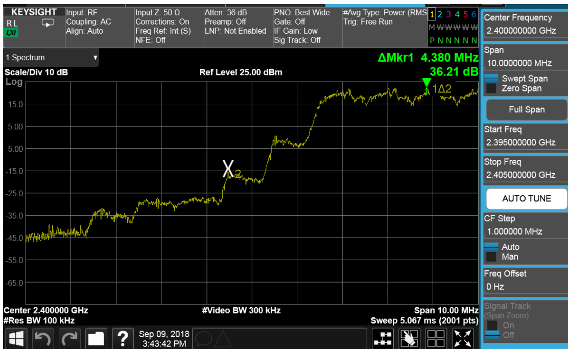
Plot 7-25. Band Edge Plot ANT 0 (Bluetooth with Hopping Enabled, 8DPSK, ePA)
