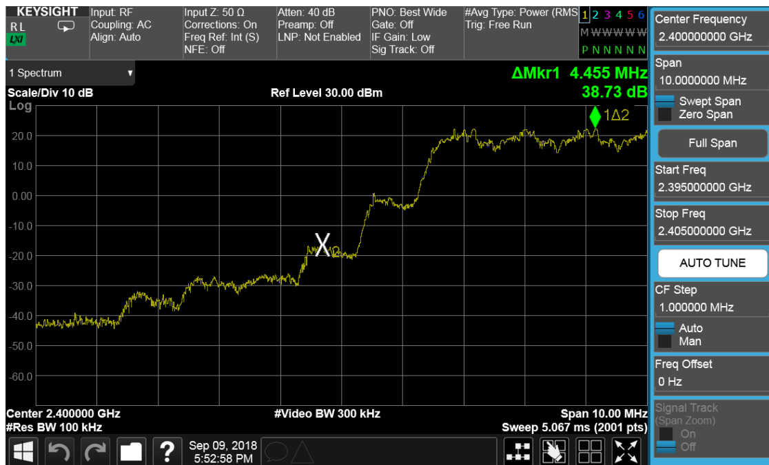
Plot 7-41. Band Edge Plot ANT 2 (Bluetooth with Hopping Enabled, 8DPSK, ePA)
