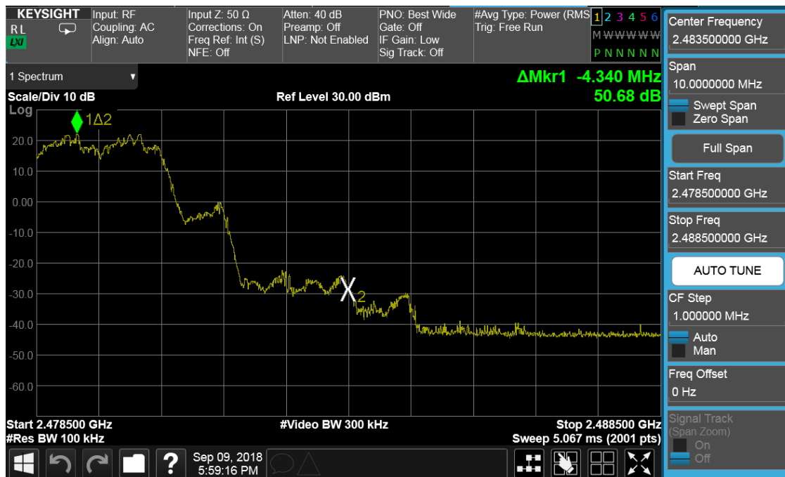
Plot 7-42. Band Edge Plot ANT 2 (Bluetooth with Hopping Enabled, 8DPSK, ePA)
