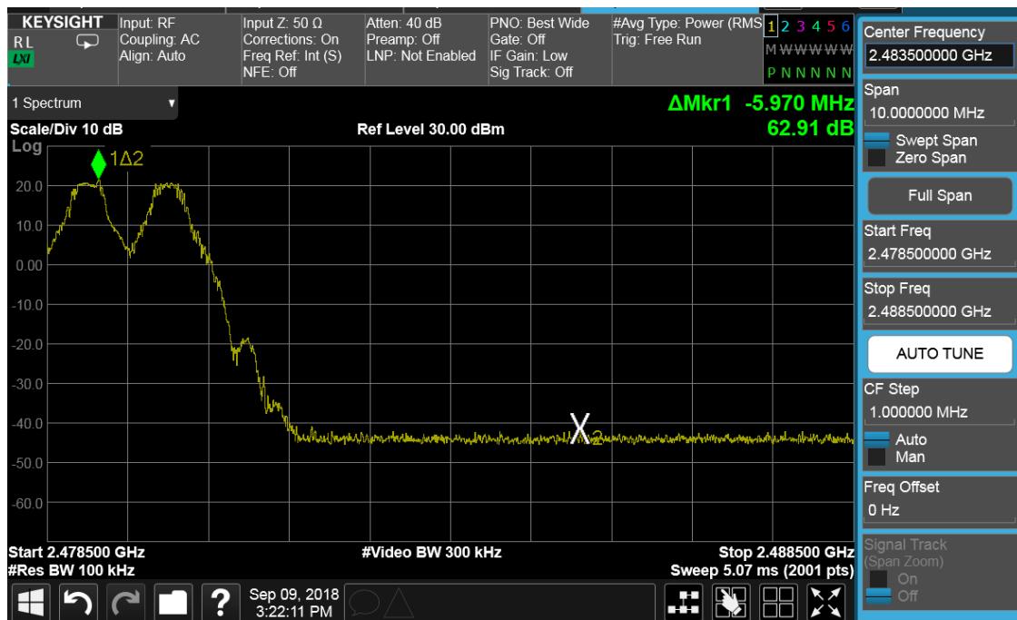
Plot 7-22. Band Edge Plot ANT 0 (Bluetooth with Hopping Enabled, GFSK, ePA)
