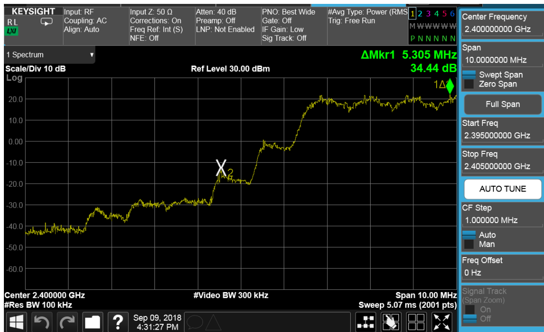
Plot 7-33. Band Edge Plot ANT 1 (Bluetooth with Hopping Enabled, 8DPSK, ePA)
