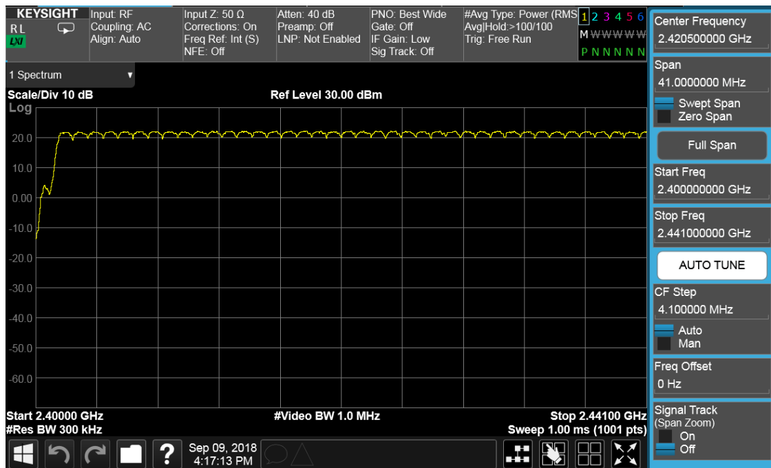
Plot 7-61. Low End Spectrum Channel Hopping Plot ANT1 (Bluetooth, 8DPSK, ePA)
