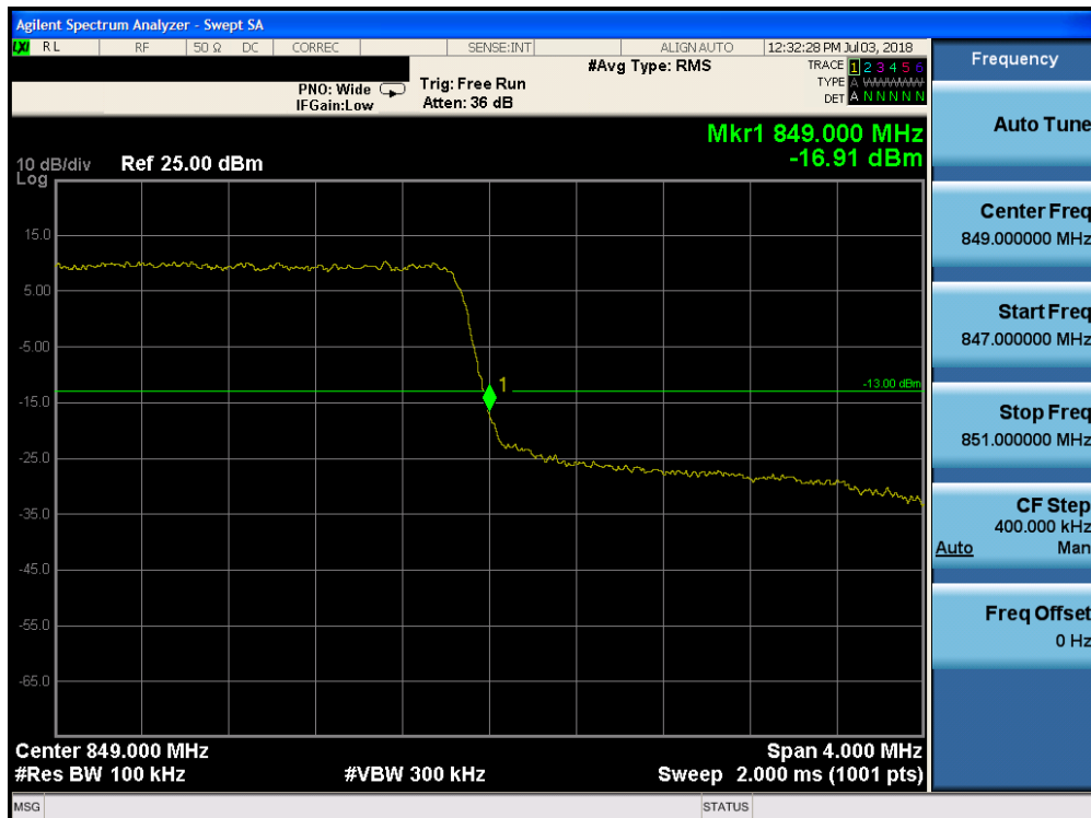
Plot 7-183. Upper Band Edge Plot (Band 26 - 3.0MHz QPSK - Full RB Configuration)
