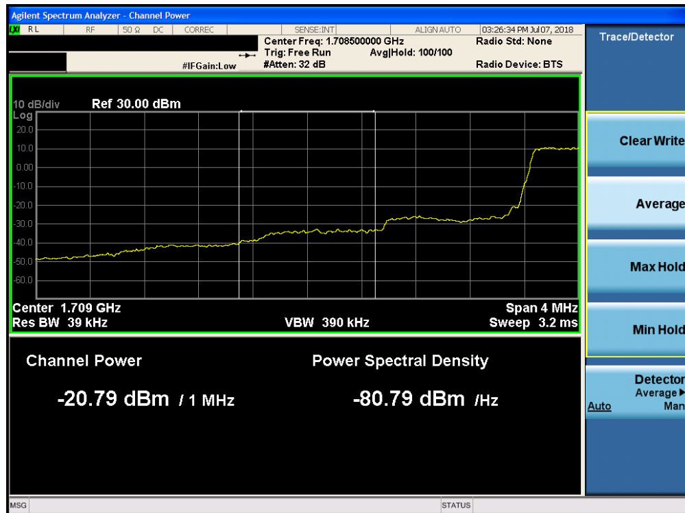
Plot 7-199. Lower Extended Band Edge Plot (Band 4 - 1.4MHz QPSK - Full RB Configuration)
