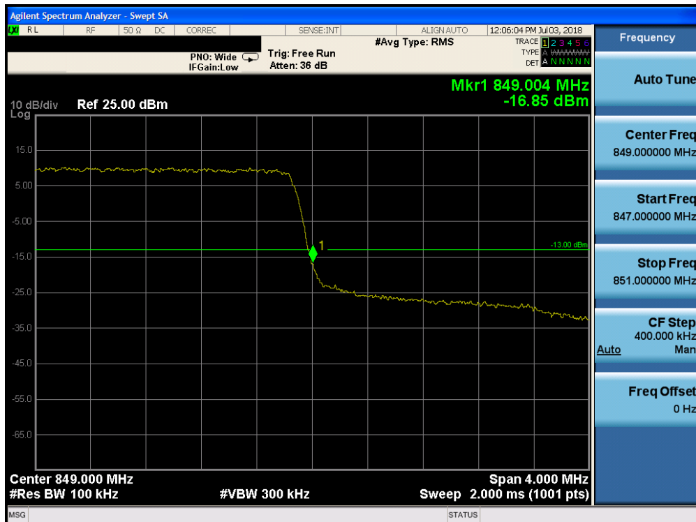
Plot 7-193. Upper Band Edge Plot (Band 5 - 3.0MHz QPSK - Full RB Configuration)
