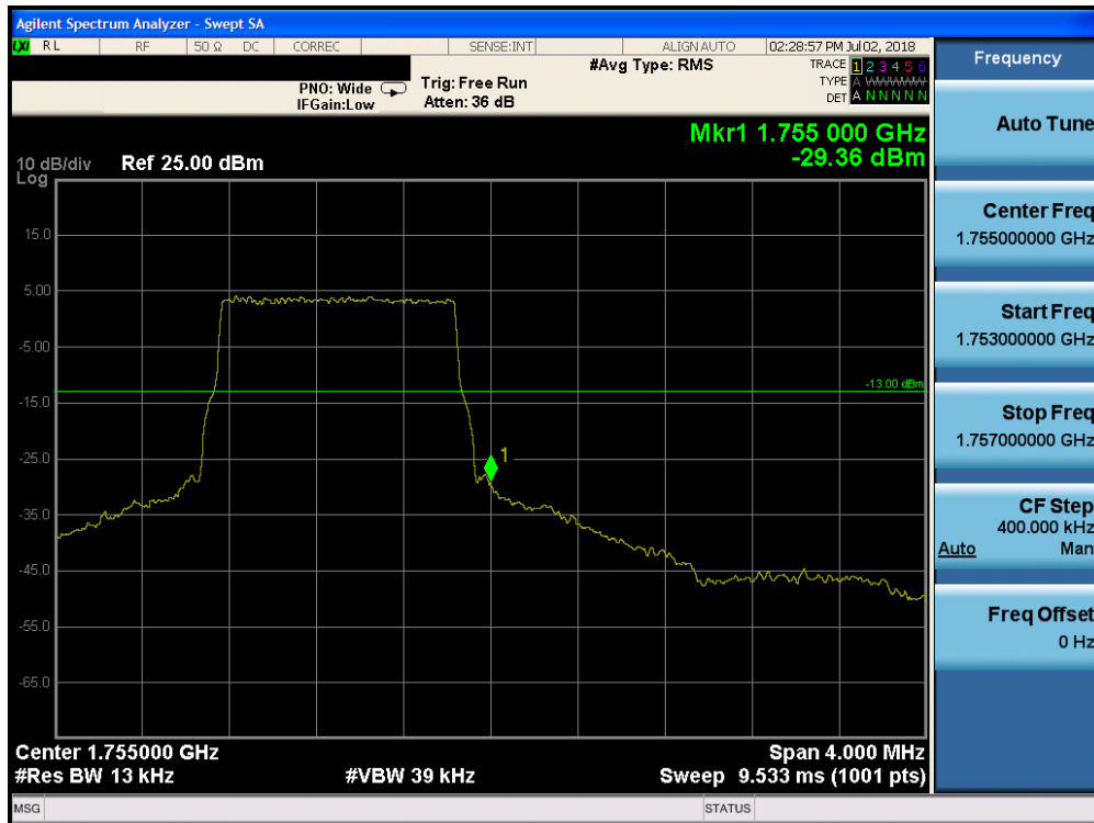
Plot 7-200. Upper Band Edge Plot (Band 4 - 1.4MHz QPSK - Full RB Configuration)
