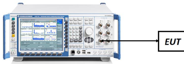
Figure 7-6. ERP/EIRP Measurement Setup
