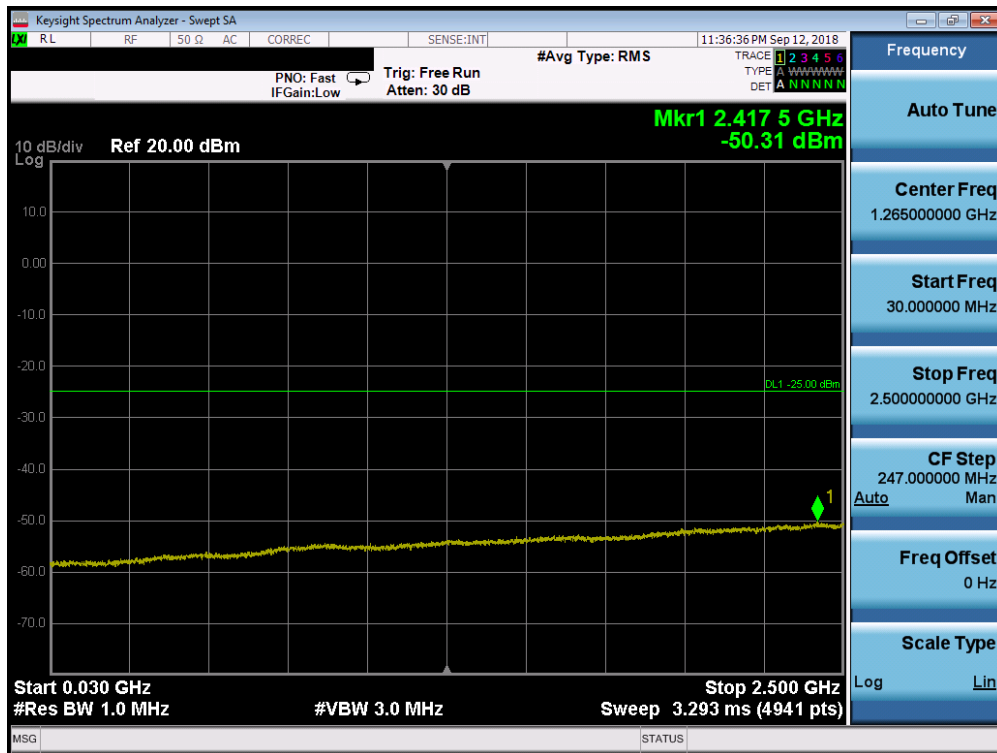
Plot 7-387. Conducted Spurious Plot (Band 7 – 20.0MHz QPSK – PCC 1/99 SCC 1/0 – Mid Channel)
