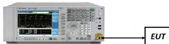
Figure 7-1. Test Instrument & Measurement Setup
