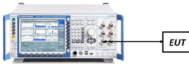
Figure 7-5. ERP/EIRP Measurement Setup
