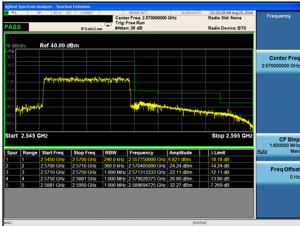
Plot 7-307. Upper ACP Plot (Band 7 – 20.0MHz QPSK – RB Size 100)
