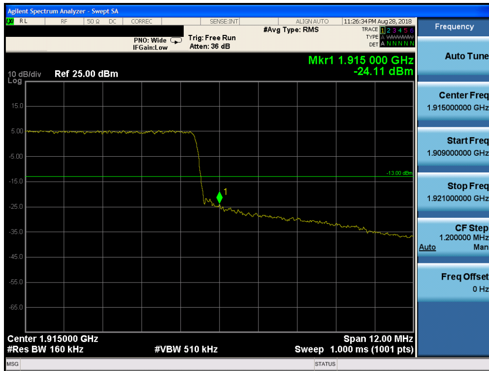
Plot 7-286. Upper Band Edge Plot (Band 25 – 15.0MHz QPSK – RB Size 75)
