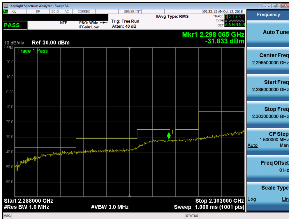
Plot 7-297. Lower Extended Band Edge Plot 2288 MHz – 2303 MHz (Band 30 – 10.0MHz QPSK – RB Size 50)
