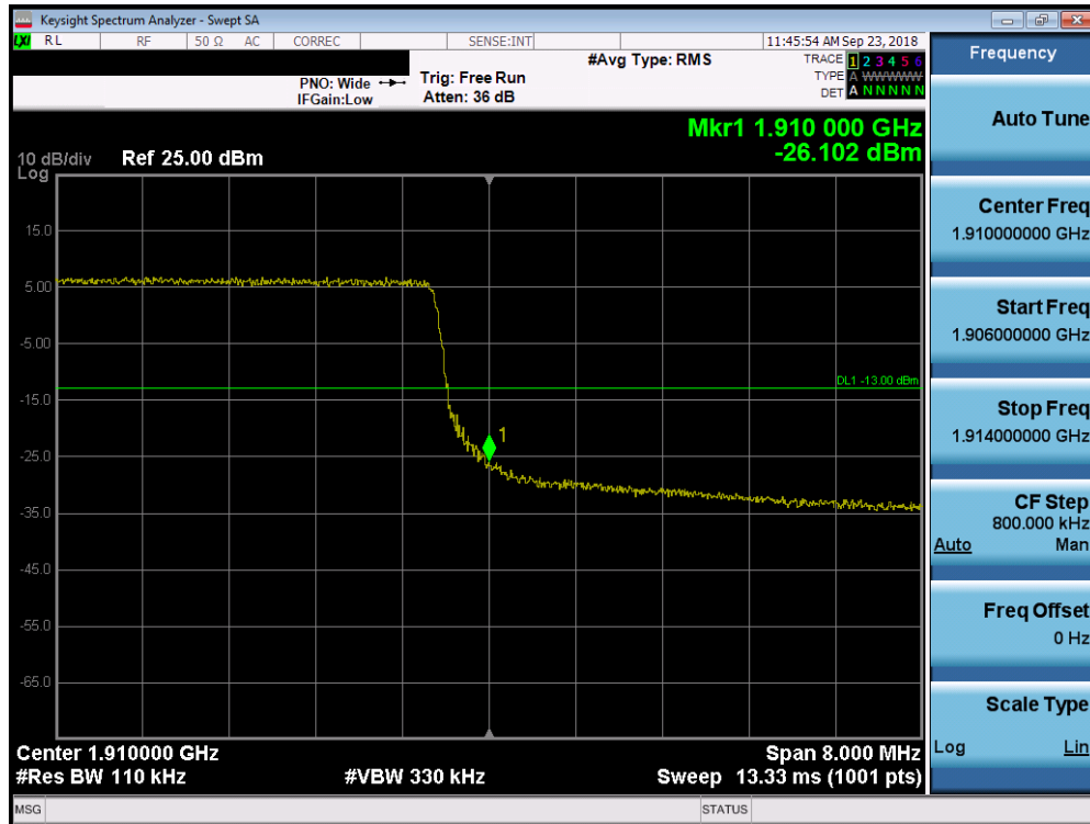
Plot 7-258. Upper Band Edge Plot (Band 2 – 10.0MHz QPSK – RB Size 50)
