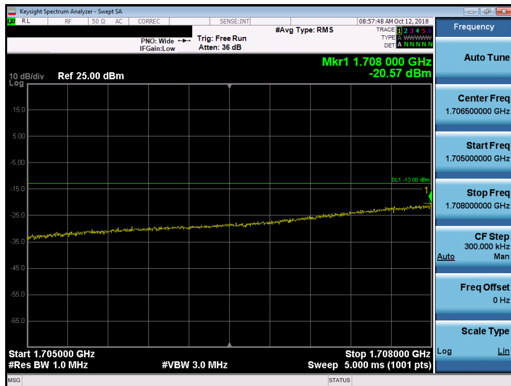
Plot 7-225. Lower Extended Band Edge Plot (Band 66 – 3.0MHz QPSK – RB Size 15)
