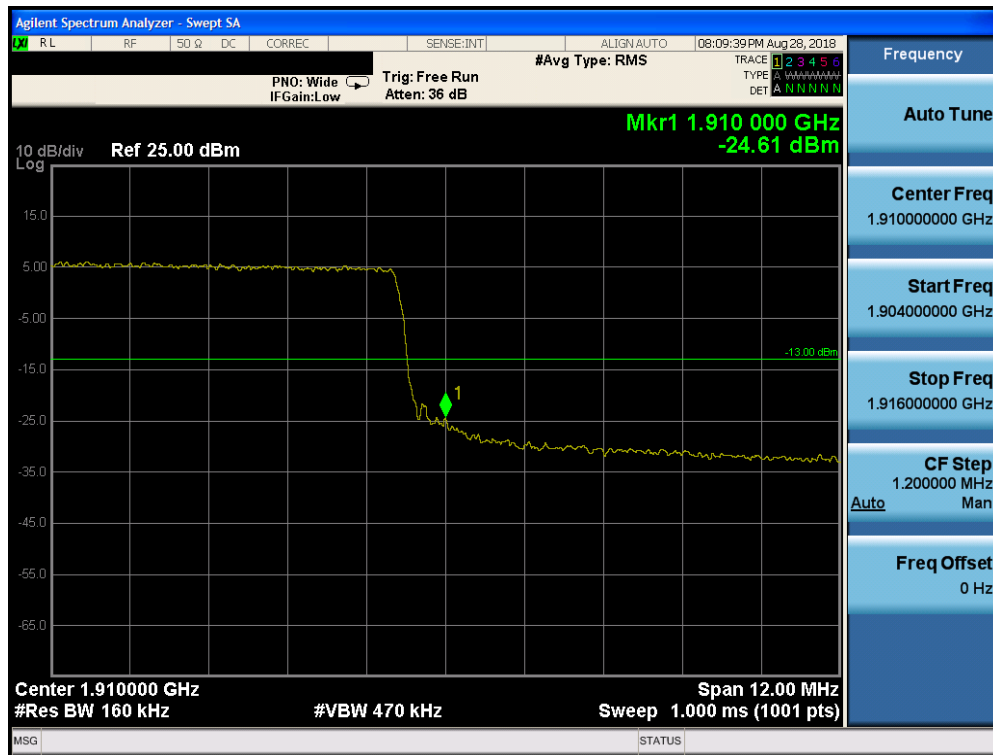
Plot 7-262. Upper Band Edge Plot (Band 2 – 15.0MHz QPSK – RB Size 75)
