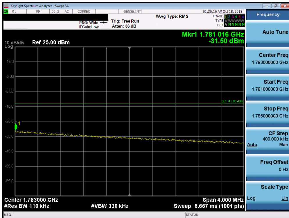
Plot 7-235. Upper Extended Band Edge Plot (Band 66 – 10.0MHz QPSK – RB Size 50)
