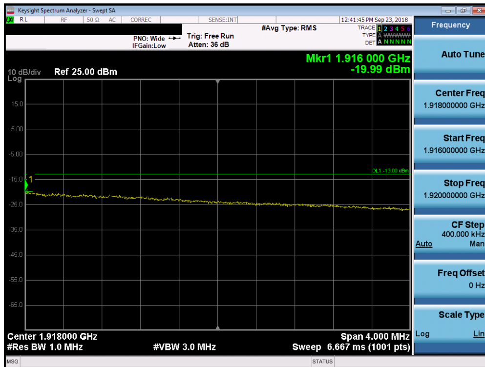
Plot 7-287. Upper Extended Band Edge Plot (Band 25 – 15.0MHz QPSK – RB Size 75)
