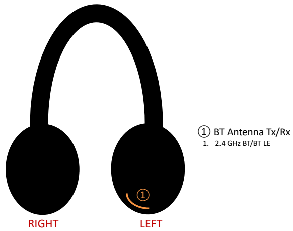
Figure F-1 DUT Antenna Locations
