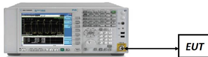
Figure 7-3. Test Instrument & Measurement Setup
