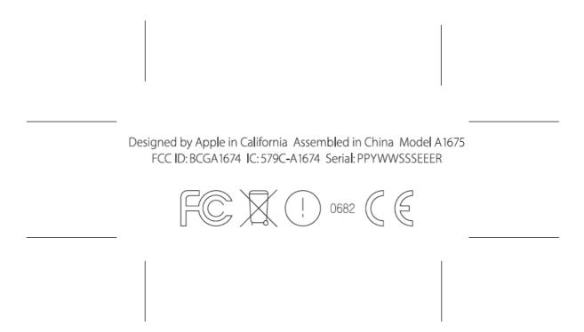
The label is etched on the rear side exterior of the device and it is always visible without using any tool.
