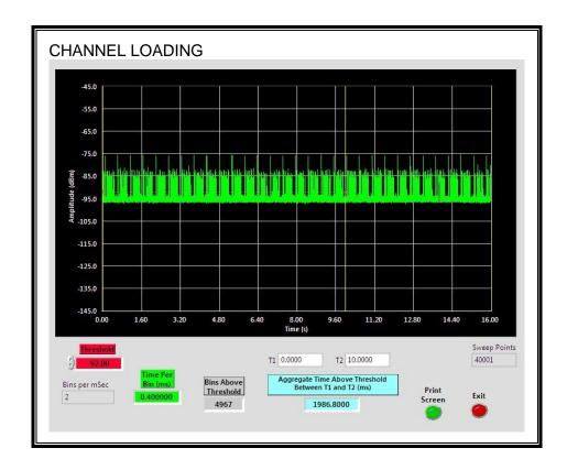
The level of traffic loading on the channel by the EUT is 19.86%
