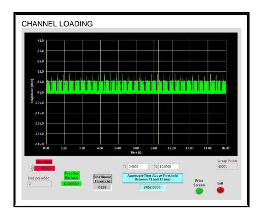
The level of traffic loading on the channel by the EUT is 24.62%
