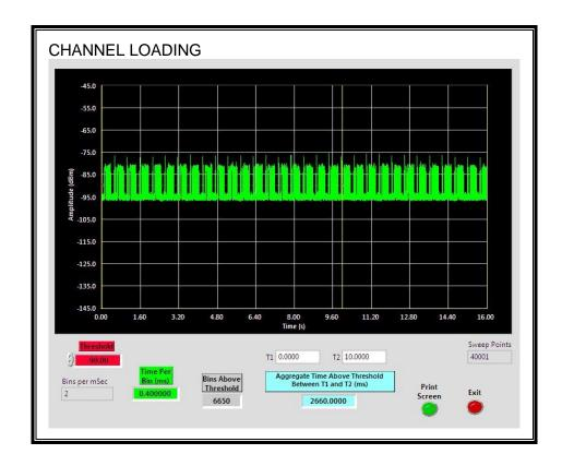
The level of traffic loading on the channel by the EUT is 26.6%
