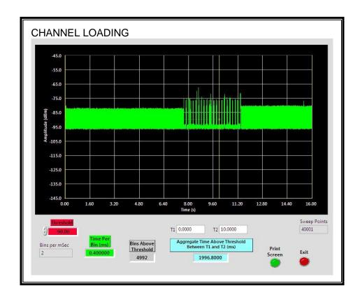
The level of traffic loading on the channel by the EUT is 19.968%
