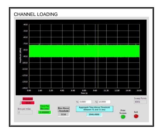
The level of traffic loading on the channel by the EUT is 20.46%
