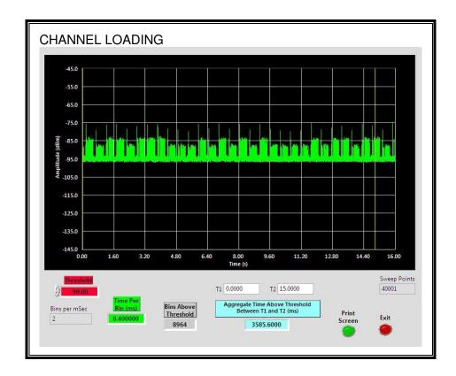
The level of traffic loading on the channel by the EUT is 35.85%
