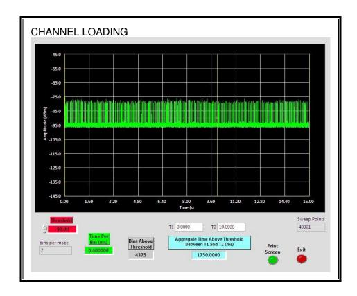
The level of traffic loading on the channel by the EUT is 17.5%
