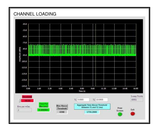
The level of traffic loading on the channel by the EUT is 17.59%
