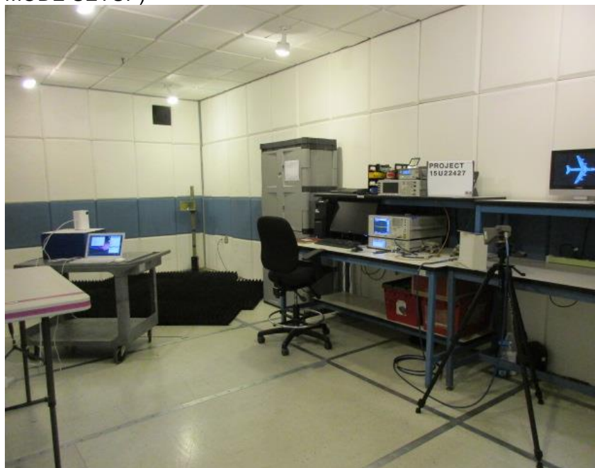
DFS FRONT PHOTO (CLIENT-TO-CLIENT COMMUNICATIONS MODE SETUP)
